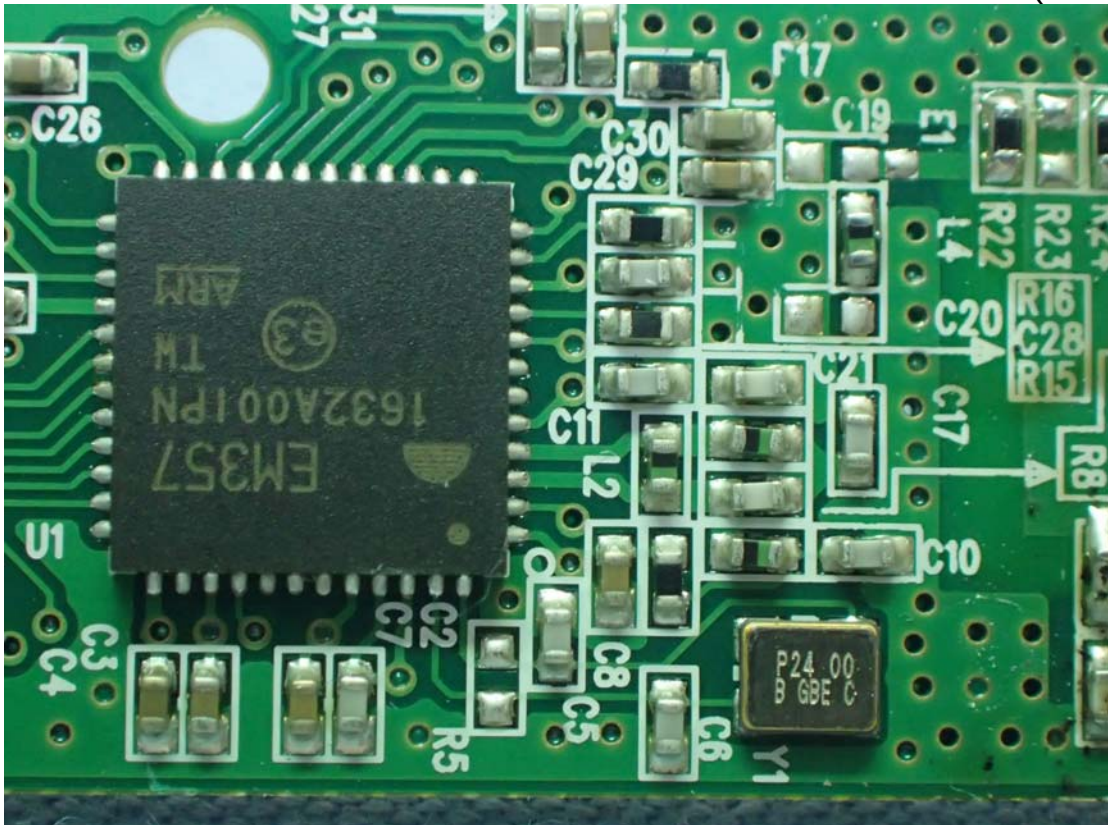
Figure 4 Internal View (RF IC)
