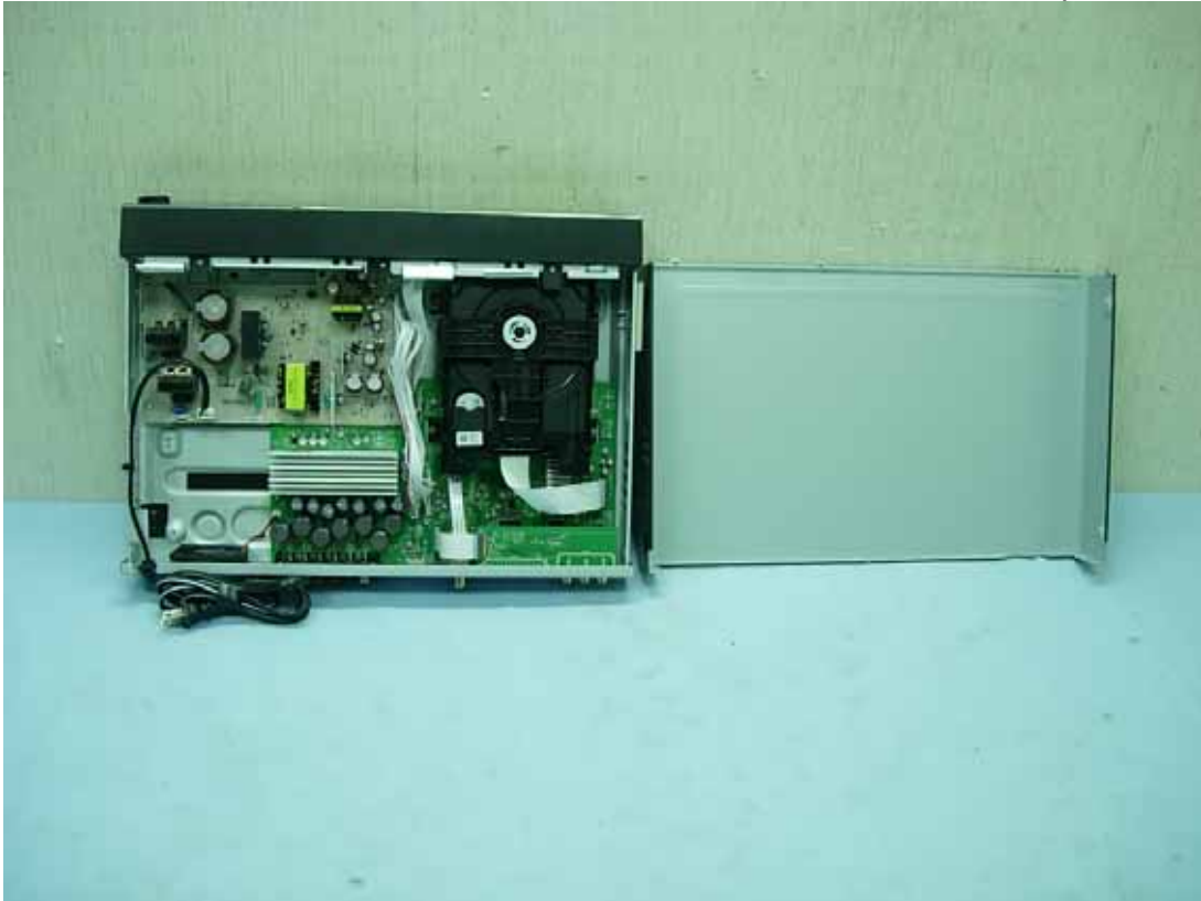
Figure 4 Internal View (Cover Removed)
