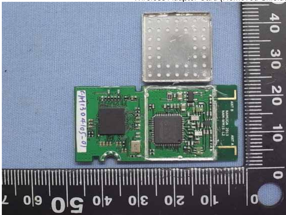
Wireless Adapter Card (Removed Shielded Case)
