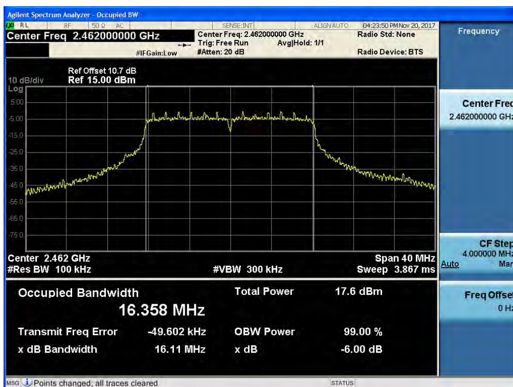
6dB Bandwidth plot (802.11g-CH 11)
