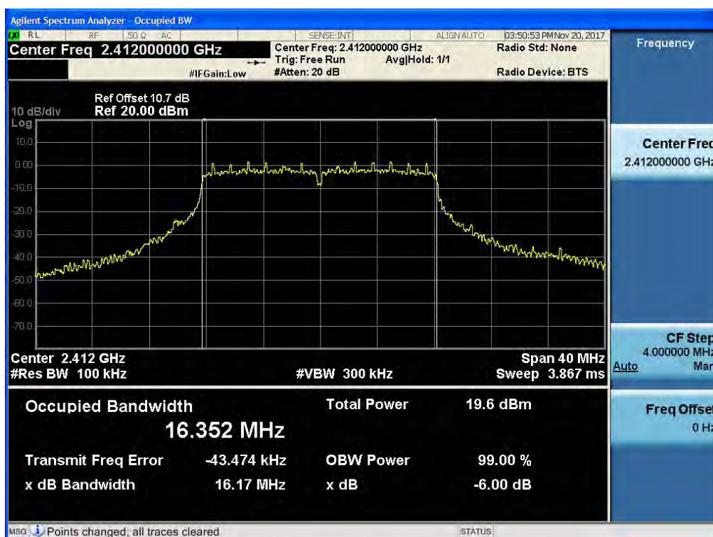
6dB Bandwidth plot (802.11g-CH 1)
