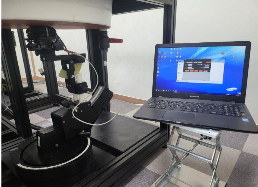
SAR Test Picture(Back), Test separation distance : 0 mm
