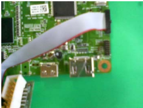
Figure 7: UART Cable connection Method
