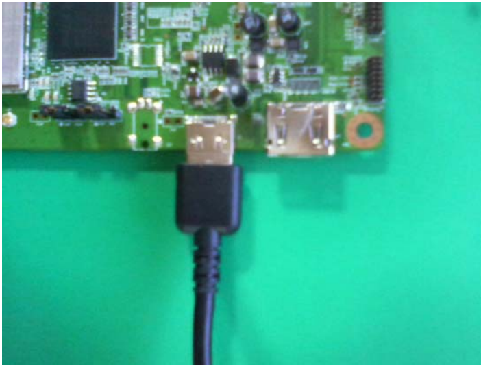
Figure 3: Control Cable connection Method
