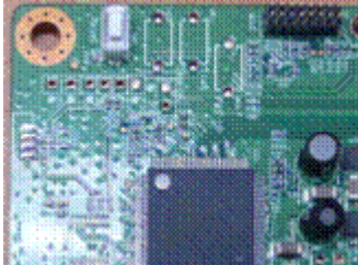
Figure 5: Reset switch location
