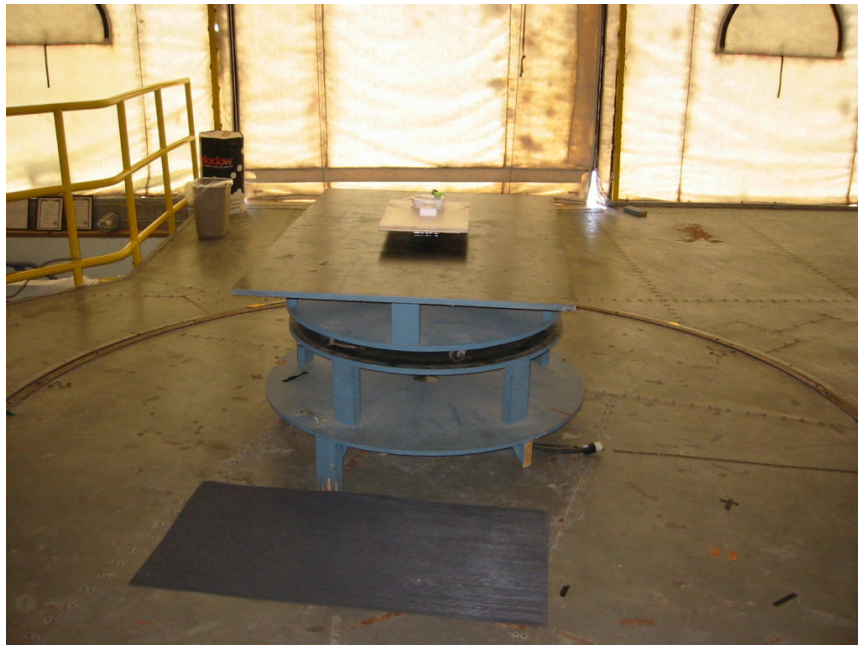
Radiated Spurious Test Setup, Back View
