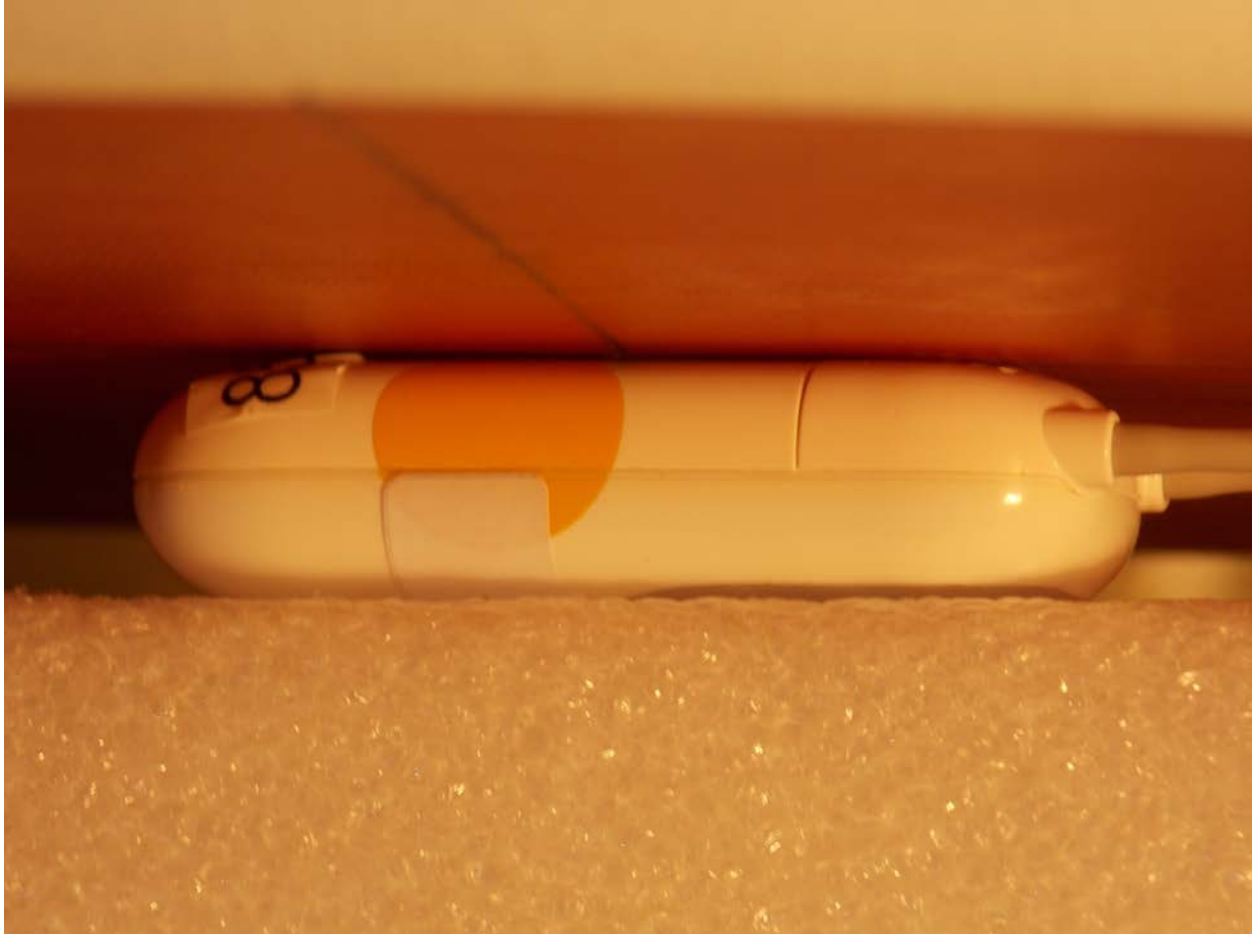
Test Position Back Extremity 0 mm Gap
