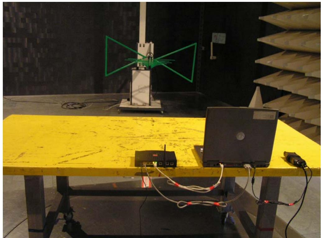
**For radiated emissions above 1GHz****FRONT VIEW**
