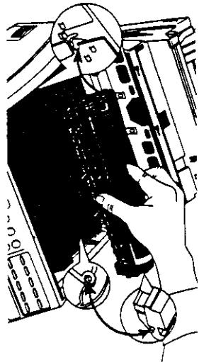
image drum are inserted correctly as shown below. Then press down firmly on both ends of the image drum until it snaps into place.
