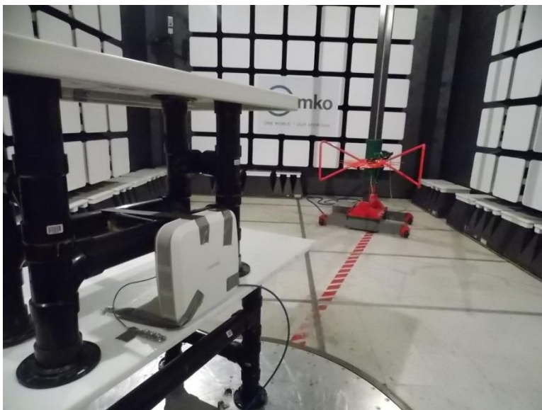
Figure 9.1-1: Radiated setup photo
