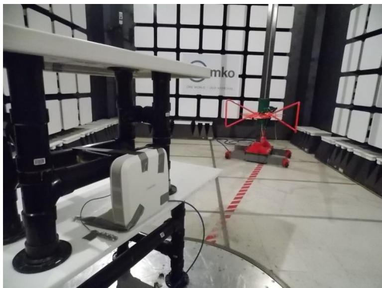
Figure 9.1-1: Radiated setup photo
