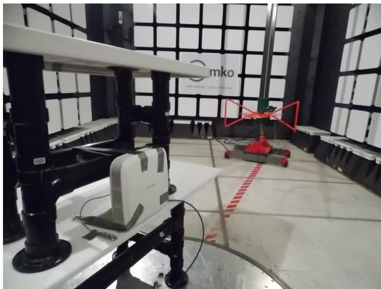
Figure 9.1-1: Radiated setup photo
