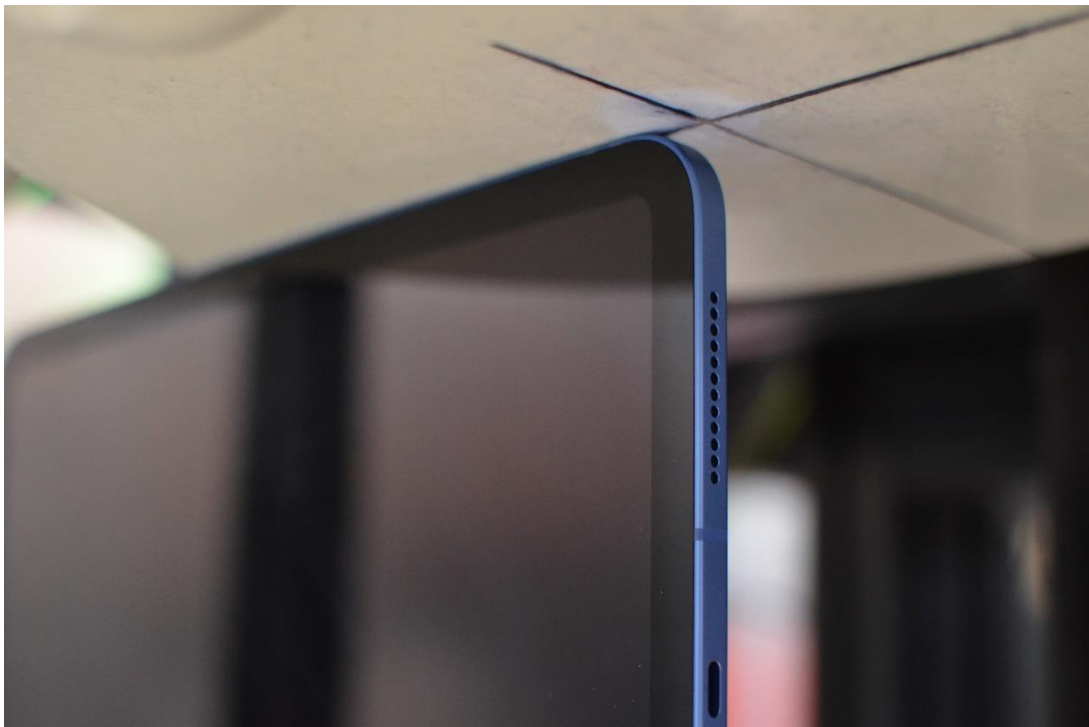
Test Setup Photo 8 – Body, Right Edge at 0.0 mm – Antenna 2a
