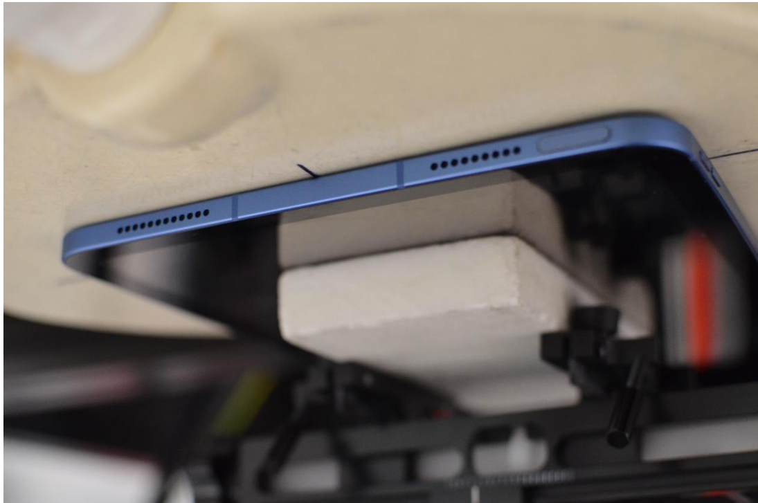
Test Setup Photo 6 – Body, Back Side at 0.0 mm – Antenna 4
