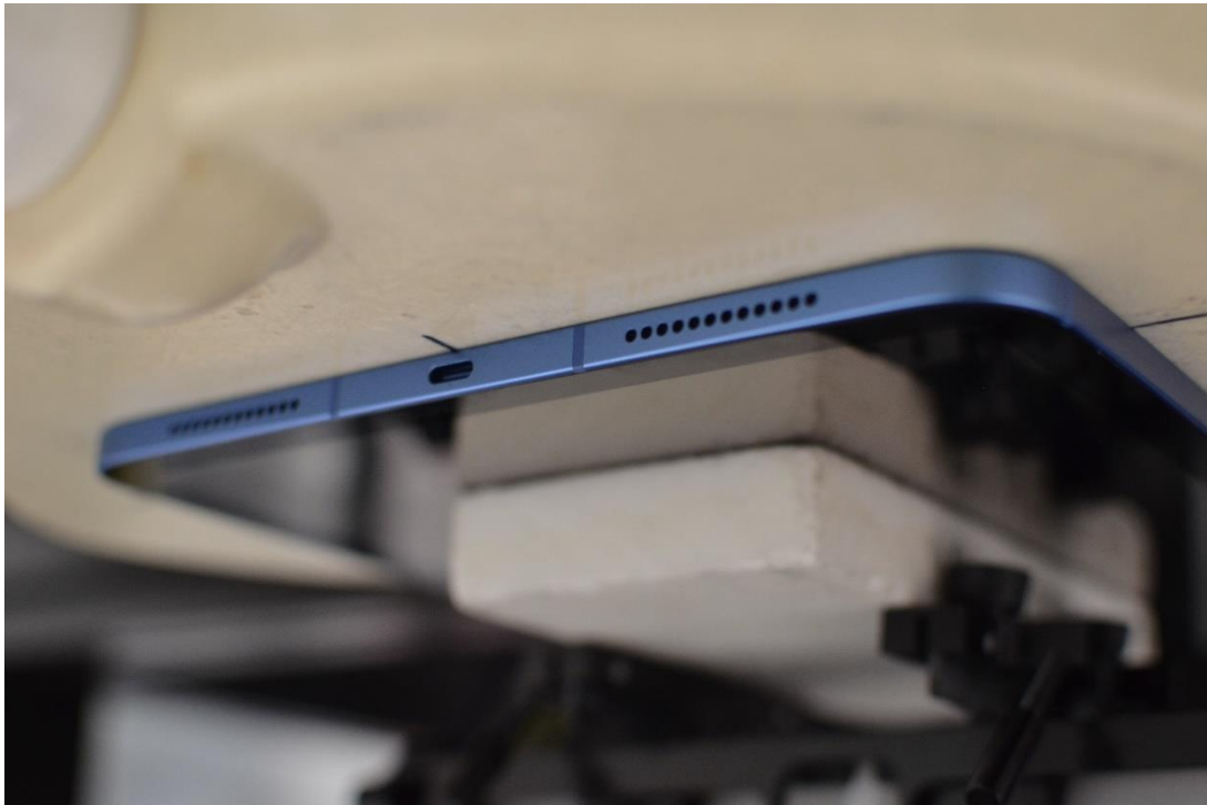
Test Setup Photo 7 – Body, Back Side at 0.0 mm – Antenna 1b/2a
