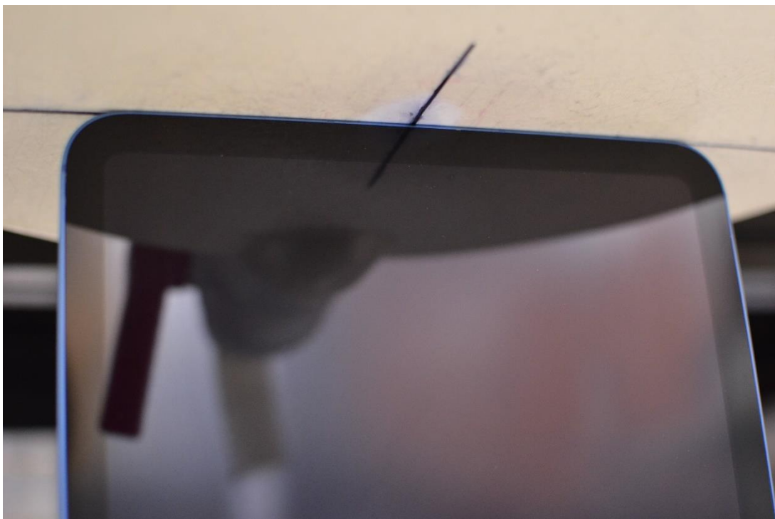
SAR Test Setup Photo 4 – Body, Bottom Edge at 0mm
