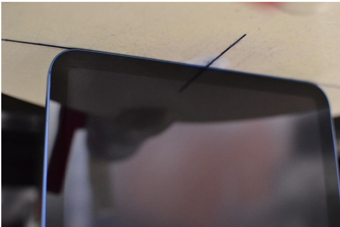
SAR Test Setup Photo 3 – Body, Top Edge at 0mm
