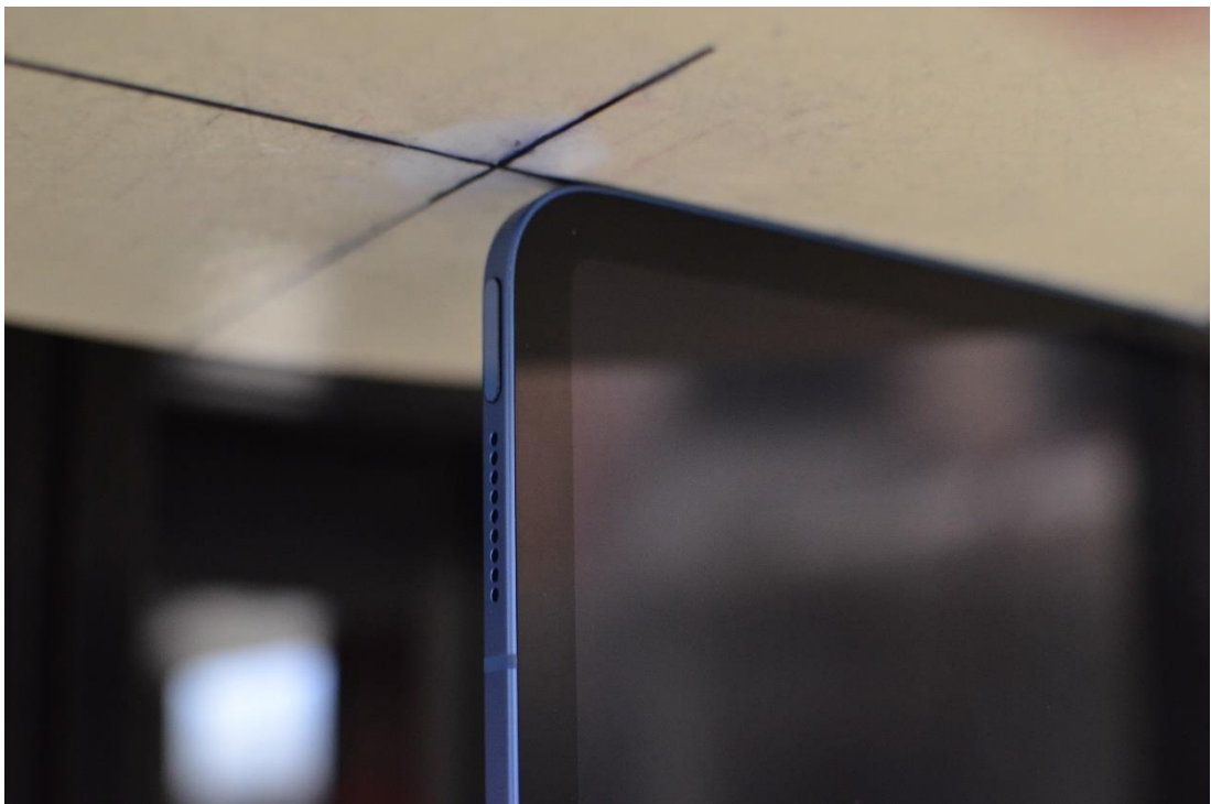
SAR Test Setup Photo 5 – Body, Right Edge at 0mm, Antennas 3a/3b/3c/4
