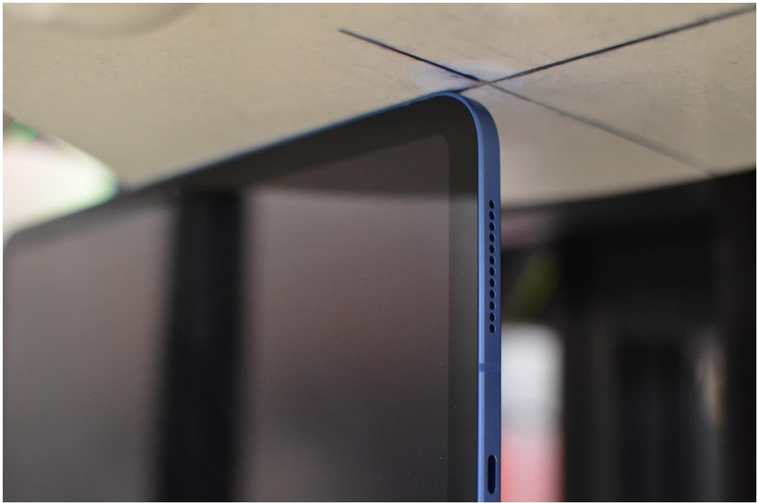
SAR Test Setup Photo 6 – Body, Right Edge at 0mm, Antennas 1a/1b/2a/2b
