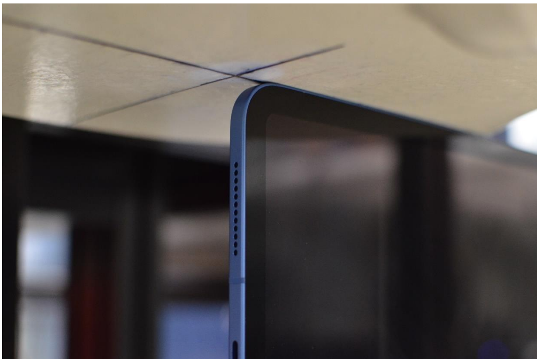
SAR Test Setup Photo 8 – Body, Left Edge at 0mm Antennas 1a/1b/2a/2b
