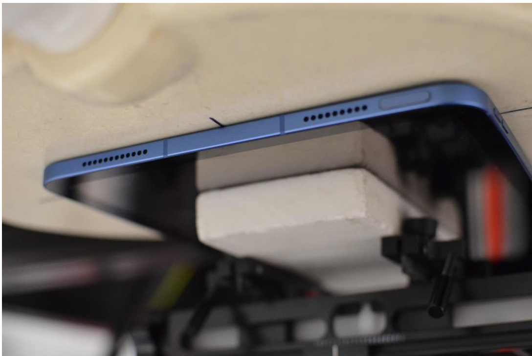
SAR Test Setup Photo 1 – Body, Back Side at 0mm, Antennas 3a/3b/3c/4
