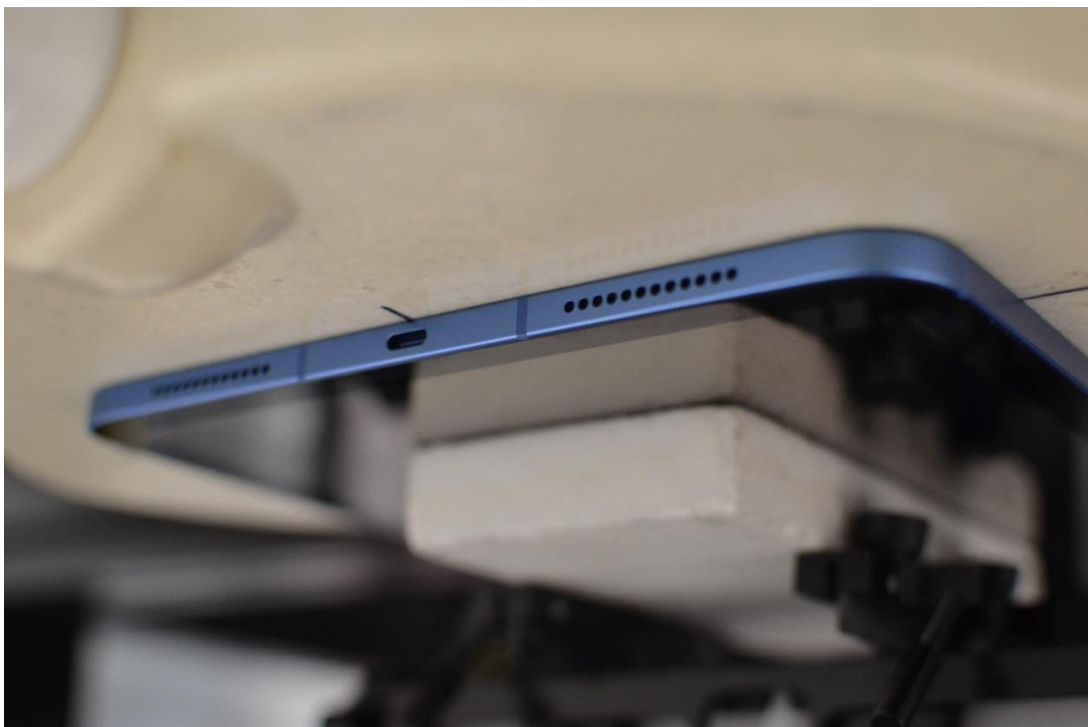
SAR Test Setup Photo 2 – Body, Back Side at 0mm, Antennas 1a/1b/2a/2b
