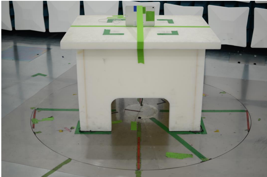
Figure 9: 30MHz-1GHz Test Setup (Front View)
