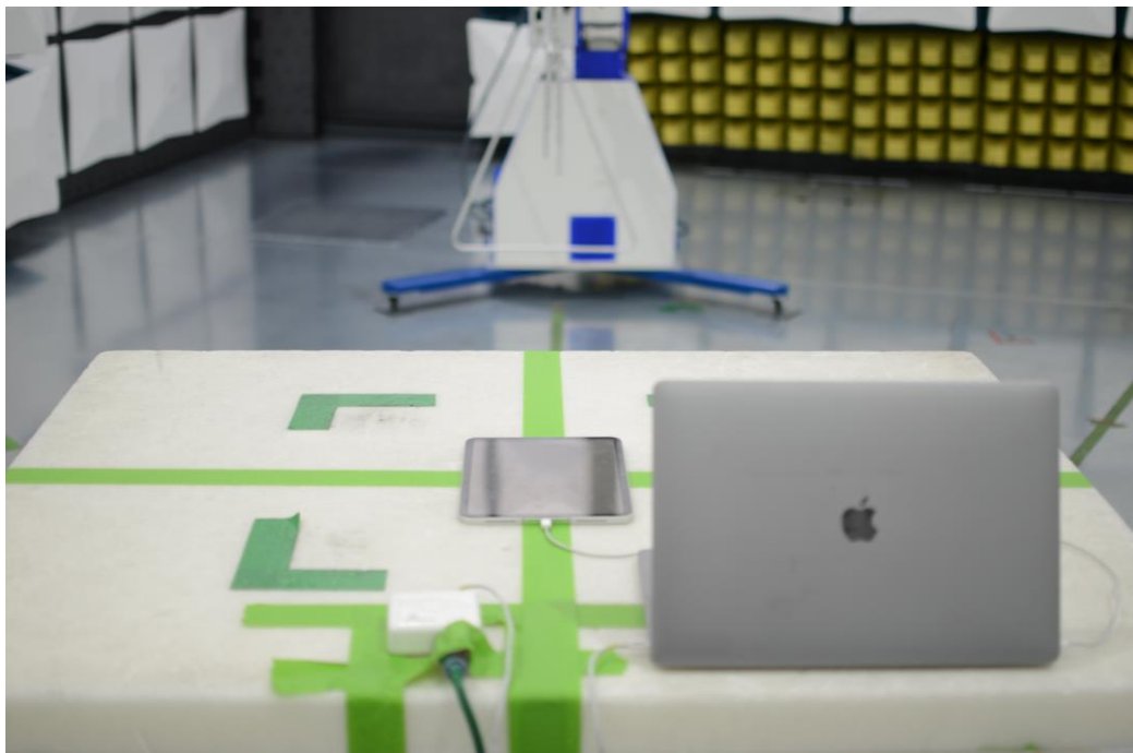
Figure 14: 30MHz-1GHz Test Setup (Rear View)
