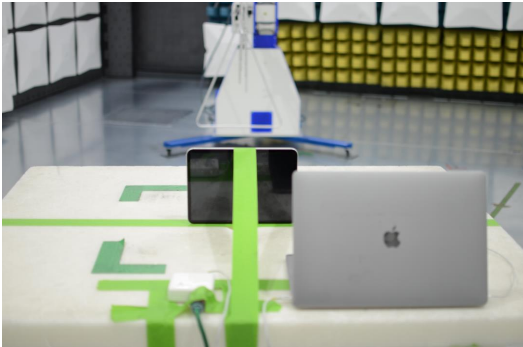
Figure 16: 30MHz-1GHz Test Setup (Rear View)
