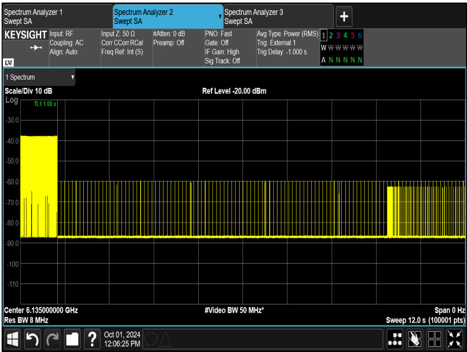
Figure 348 - U-NII-5, Maximum Bandwidth (AWGN Low), OFF Level
