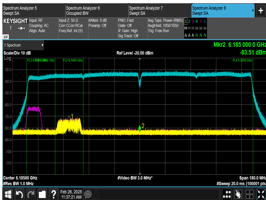
Figure 363 – Frequency Domain Plot of Channel 47 (6185 MHz) Shutdown
