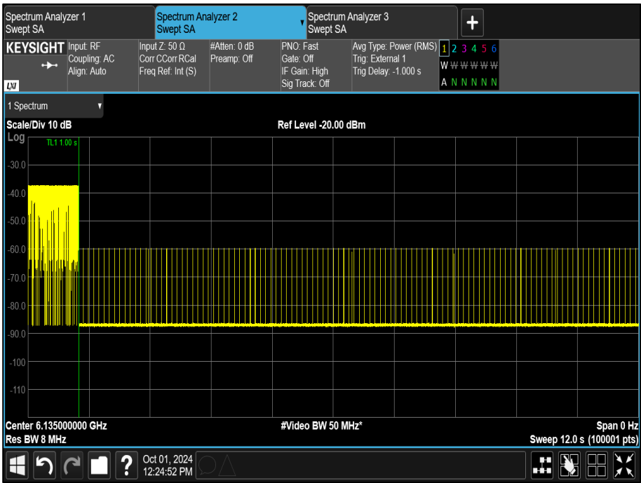
Figure 350 - U-NII-5, Maximum Bandwidth (AWGN High), OFF Level
