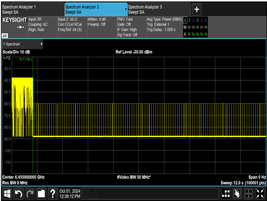
Figure 353 - U-NII-6, Maximum Bandwidth (AWGN Mid), OFF Level
