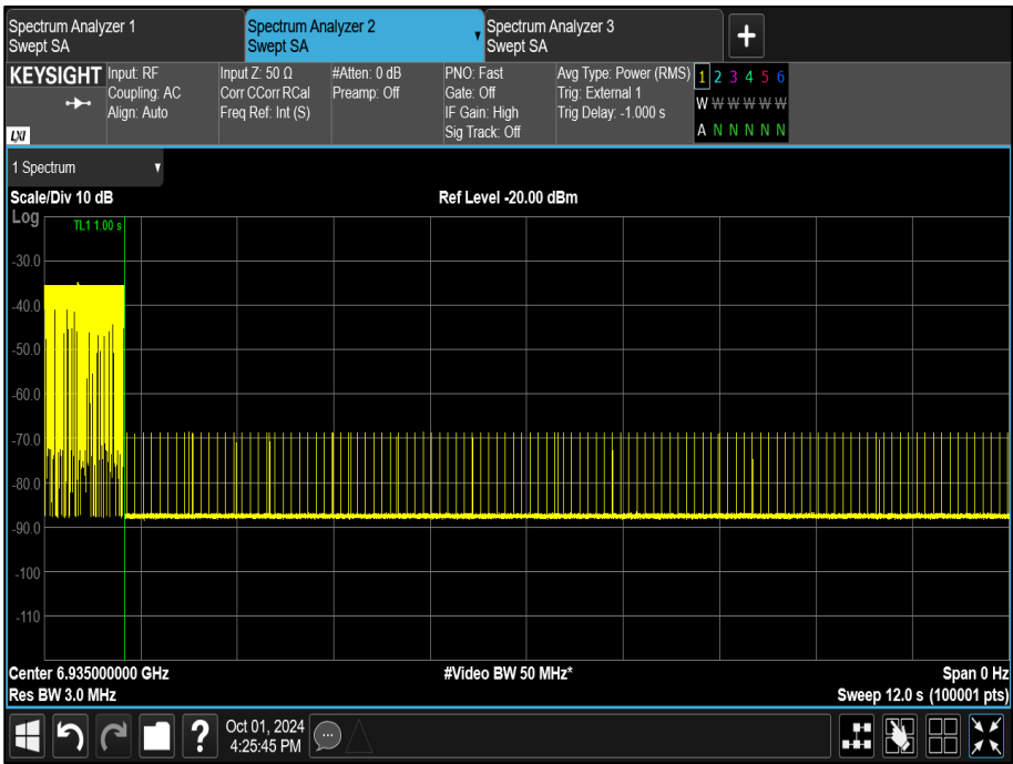
Figure 360 - U-NII-8, Maximum Bandwidth (AWGN Low), OFF Level
