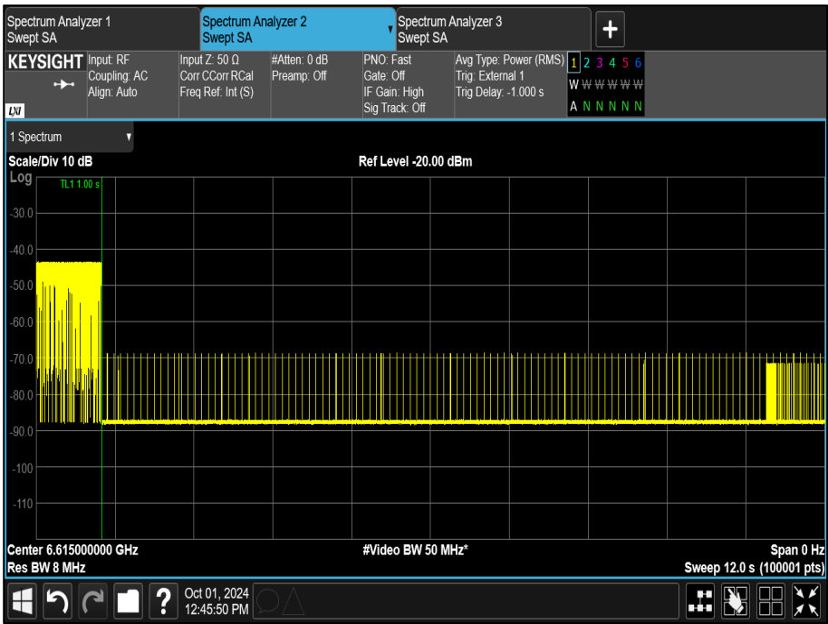
Figure 356 - U-NII-7, Maximum Bandwidth (AWGN Low), OFF Level
