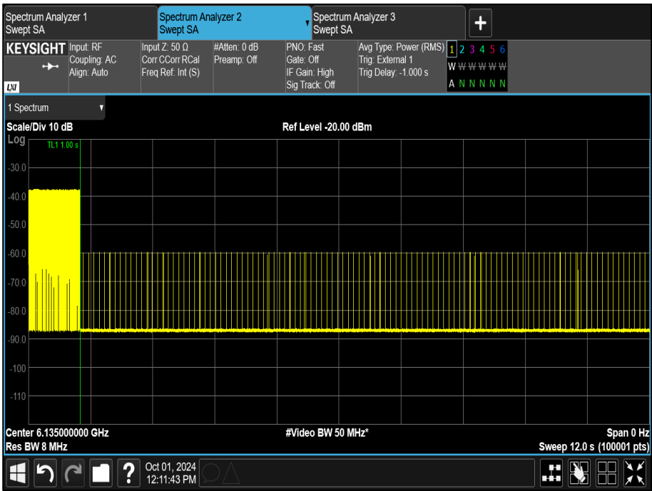
Figure 349 - U-NII-5, Max Maximum Bandwidth (AWGN Mid), OFF Level
