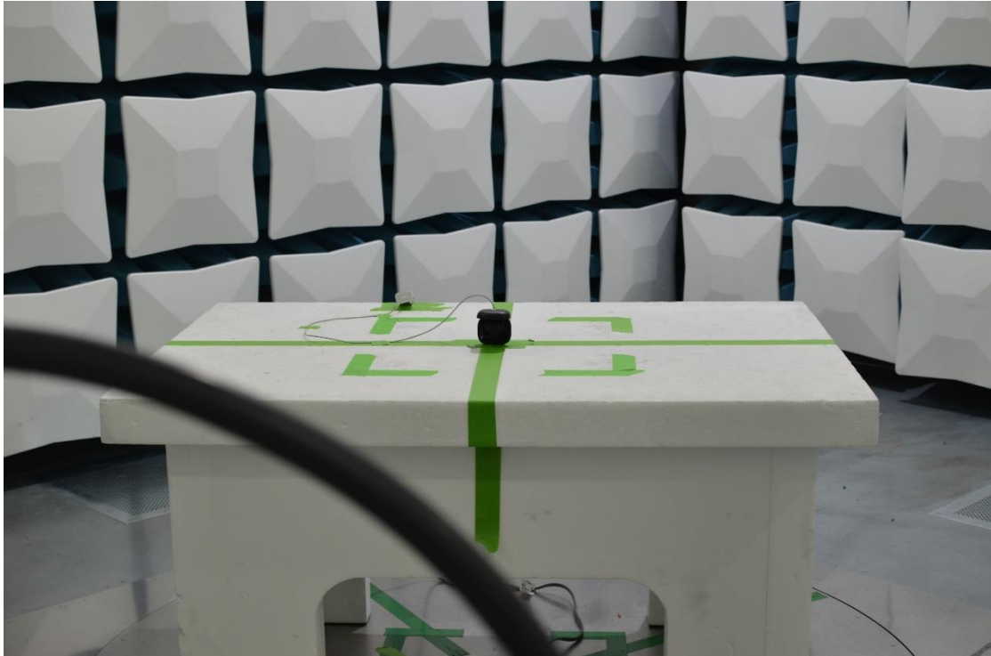
Figure 25: 9kHz-30MHz Test Setup (Front View)
