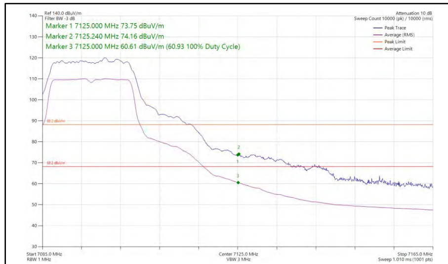
Figure 104 - 802.11a, SISO, Core 0 - 7095 MHz Band Edge Frequency 7125 MHz
