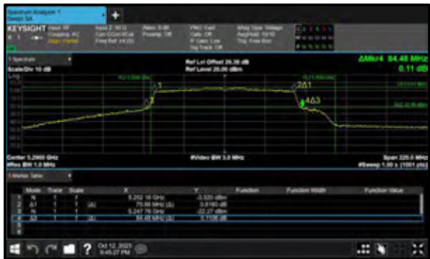
Figure 319 - 802.11ac VHT80 Minimum 99% OBW
