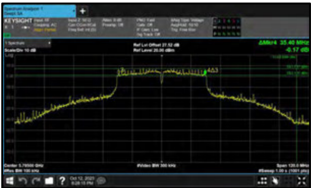
Figure 275 - 802.11n HT40 Minimum 6 dB EBW
