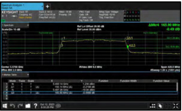
Figure 294 - 802.11ac VHT160 Maximum 99% OBW
