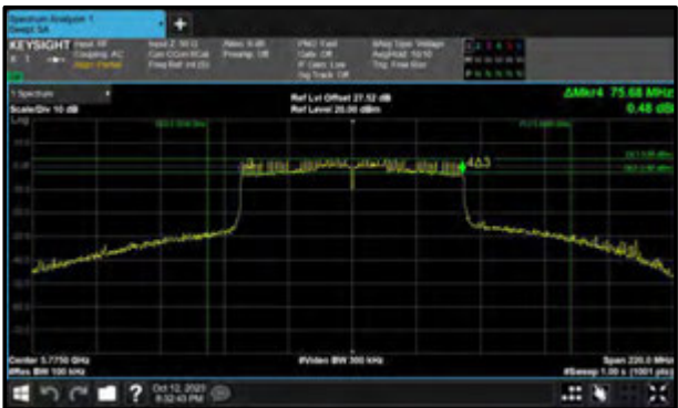
Figure 277 - 802.11ac VHT80 Minimum 6 dB EBW
