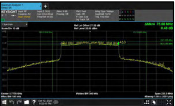
Figure 278 - 802.11ac VHT80 Maximum 6 dB EBW
