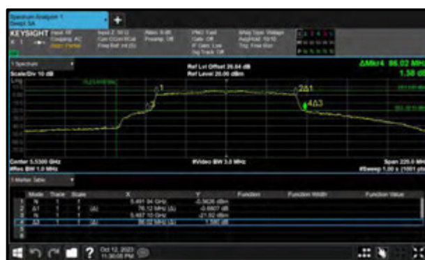
Figure 348 - 802.11ac VHT80 Maximum 99% OBW
