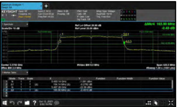
Figure 322 - 802.11ac VHT160 Maximum 99% OBW
