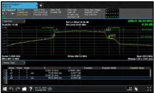
Figure 291 - 802.11ac VHT80 Minimum 99% OBW
