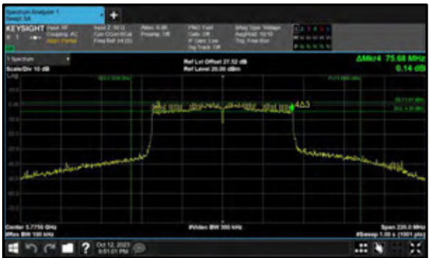
Figure 307 - 802.11ac VHT80 Minimum 6 dB EBW
