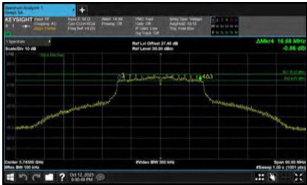
Figure 303 - 802.11n HT20 Minimum 6 dB EBW
