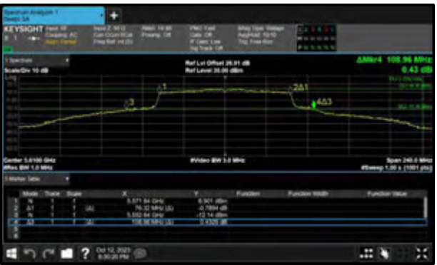
Figure 292 - 802.11ac VHT80 Maximum 99% OBW
