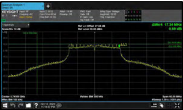
Figure 332 - 802.11n HT20 Maximum 6 dB EBW
