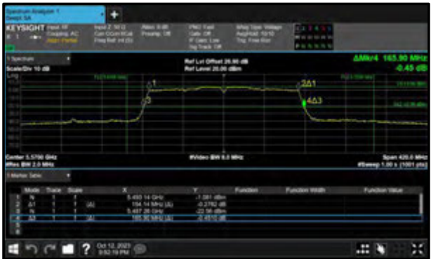
Figure 321 - 802.11ac VHT160 Minimum 99% OBW
