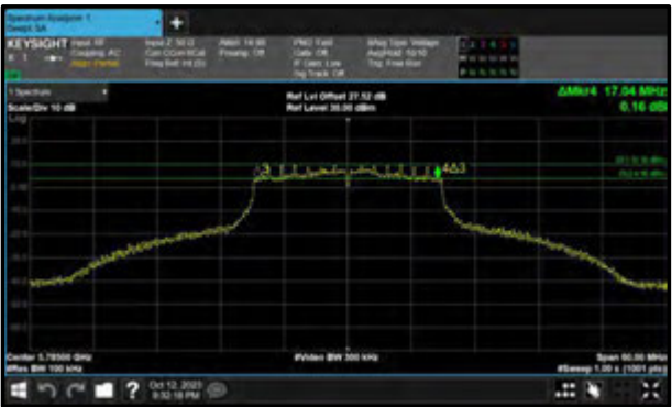
Figure 304 - 802.11n HT20 Maximum 6 dB EBW
