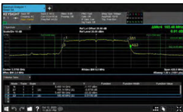
Figure 350 - 802.11ac VHT160 Maximum 99% OBW
