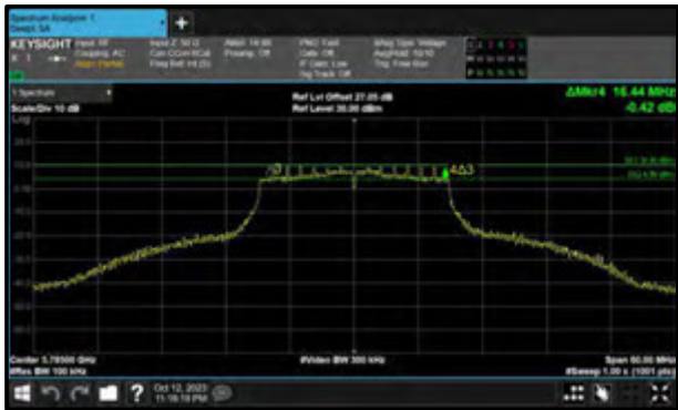
Figure 331 - 802.11n HT20 Minimum 6 dB EBW
