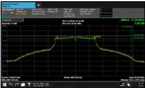
Figure 274 - 802.11n HT20 Maximum 6 dB EBW
