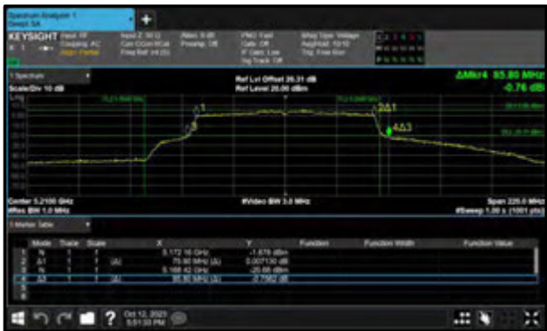
Figure 320 - 802.11ac VHT80 Maximum 99% OBW
