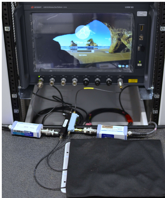
Test Setup Photo 4 – Conducted Test Setup (Figure 5-1c)
