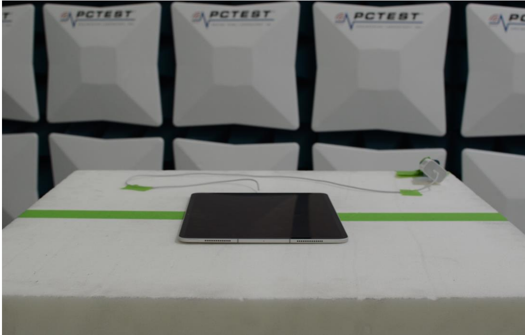
Figure 5: 1-18GHz Test Setup (Front View)
