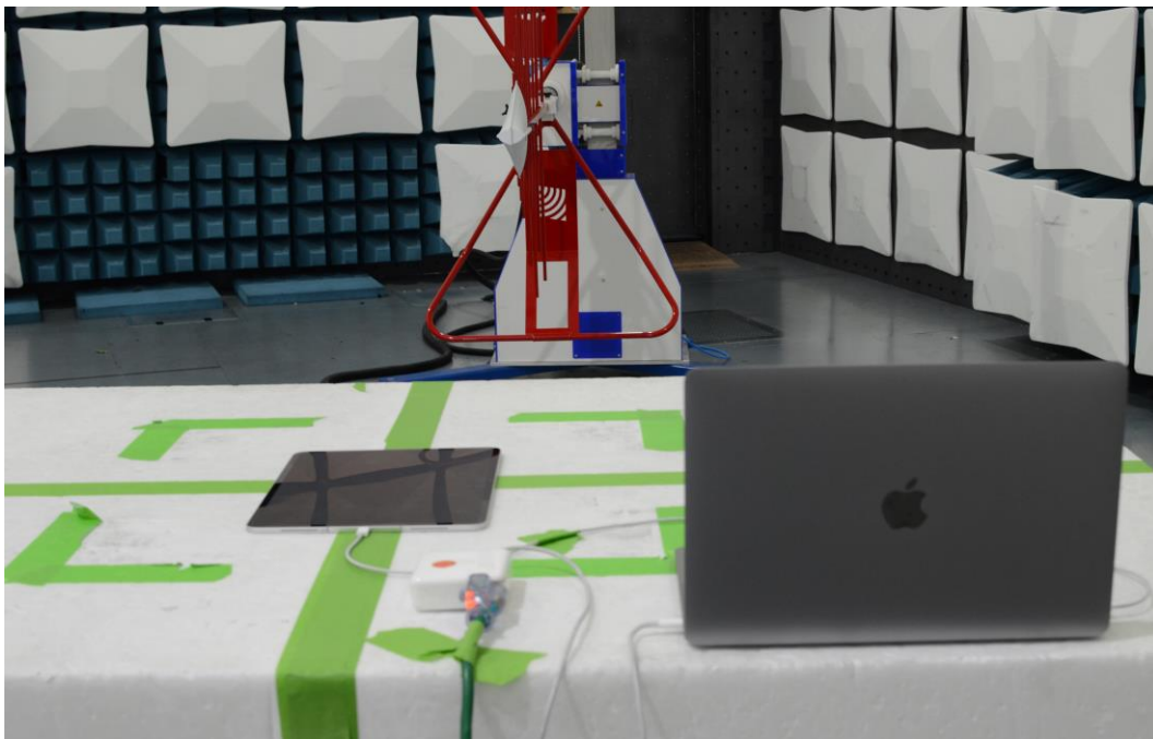
Figure 18: 30MHz-1GHz Test Setup (Rear View)
