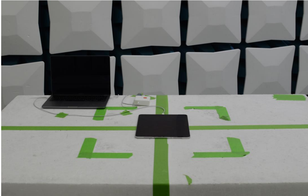
Figure 17: 30MHz-1GHz Test Setup (Front View)
