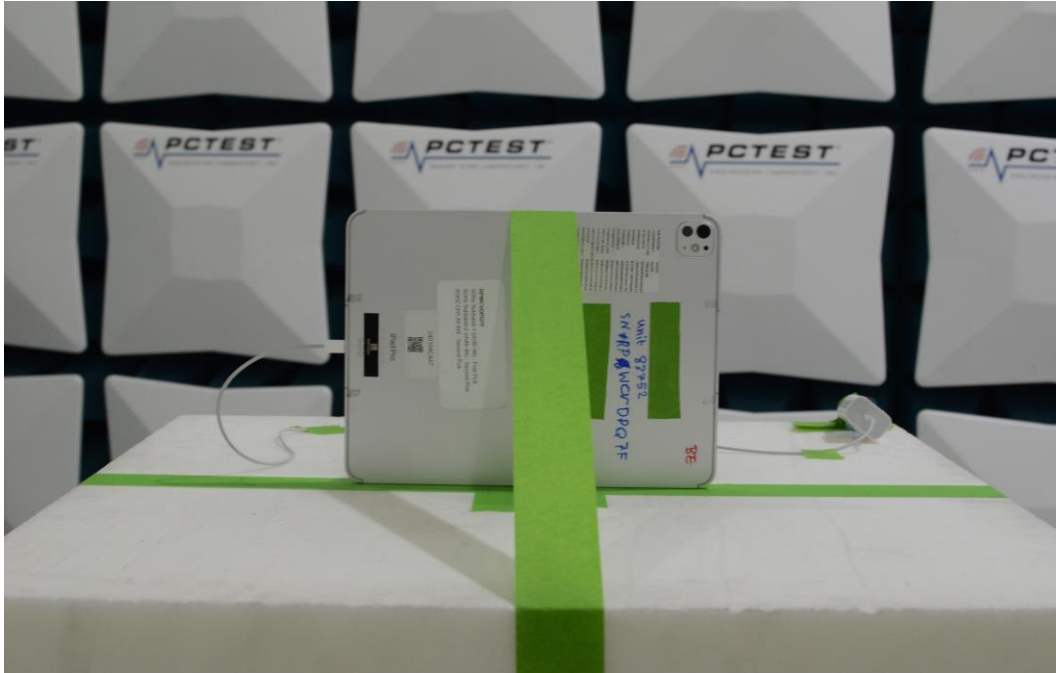
Figure 7: 1-18GHz Test Setup (Front View)
