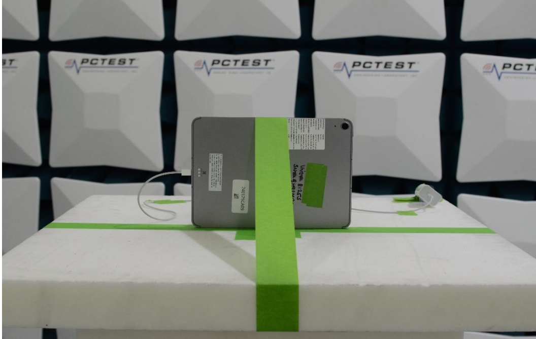
Figure 7: 1-18GHz Test Setup (Front View)
