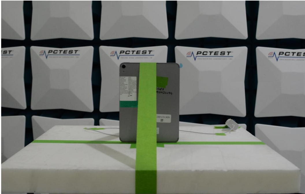
Figure 9: 1-18GHz Test Setup (Front View)
