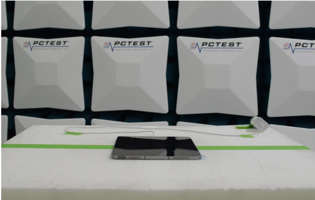
Figure 5: 1-18GHz Test Setup (Front View)
