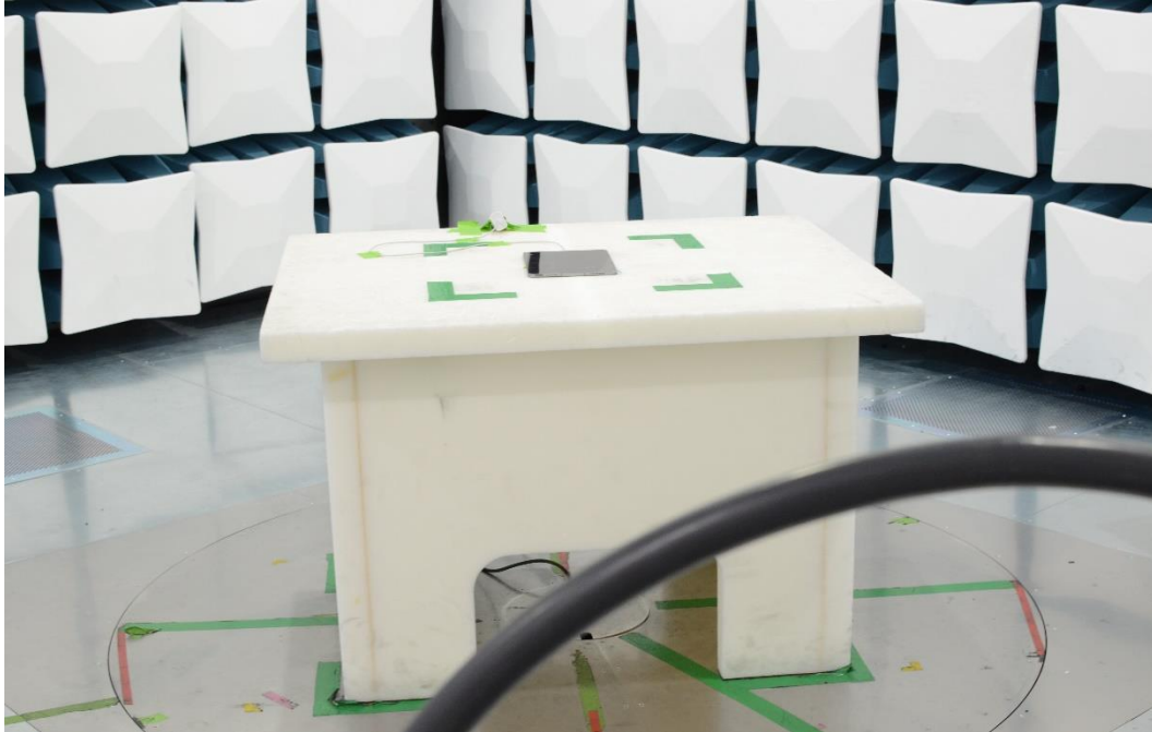
Figure 23: 9kHz-30MHz Test Setup (Front View)
