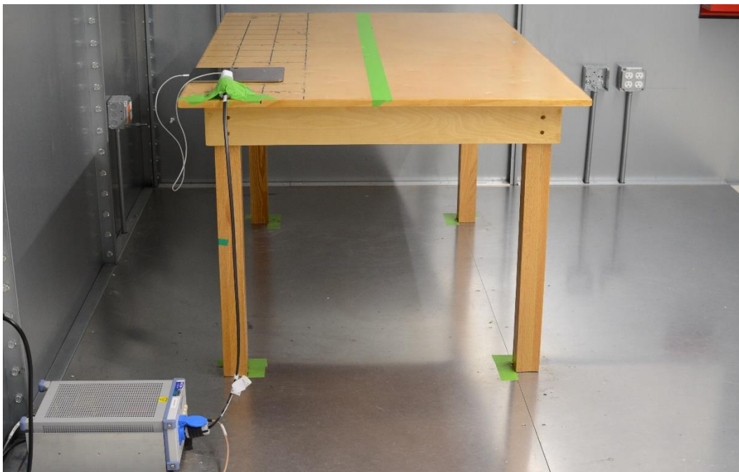
Figure 2: AC Line Conducted Emissions (Side View)
