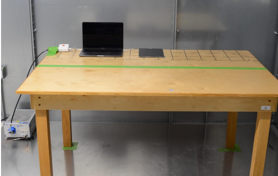
Figure 3: AC Line Conducted Emissions (Front View)
