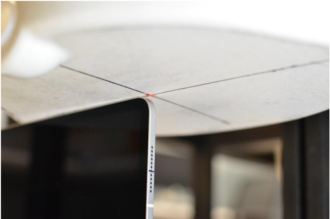
Test Setup Photo 10 – Body, Left Edge at 0.0 cm – Antenna 4
