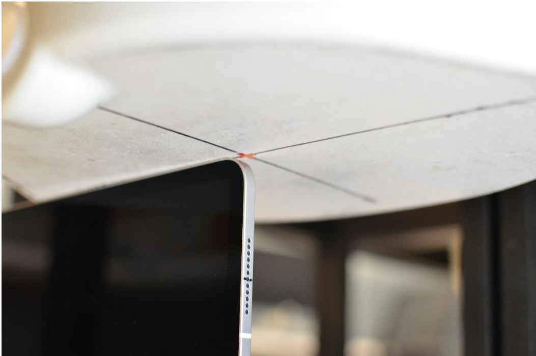
Test Setup Photo 9 – Body, Right Edge at 0.0 cm – Antenna 2
