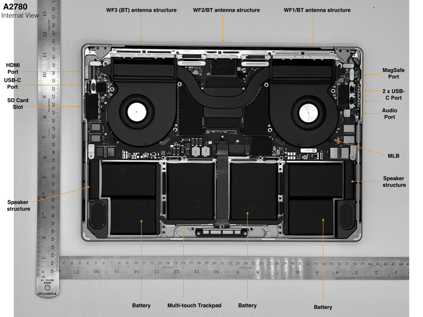
WF1/BT, WF2/BT, WF3 (BT) antenna structure and feed-Front
