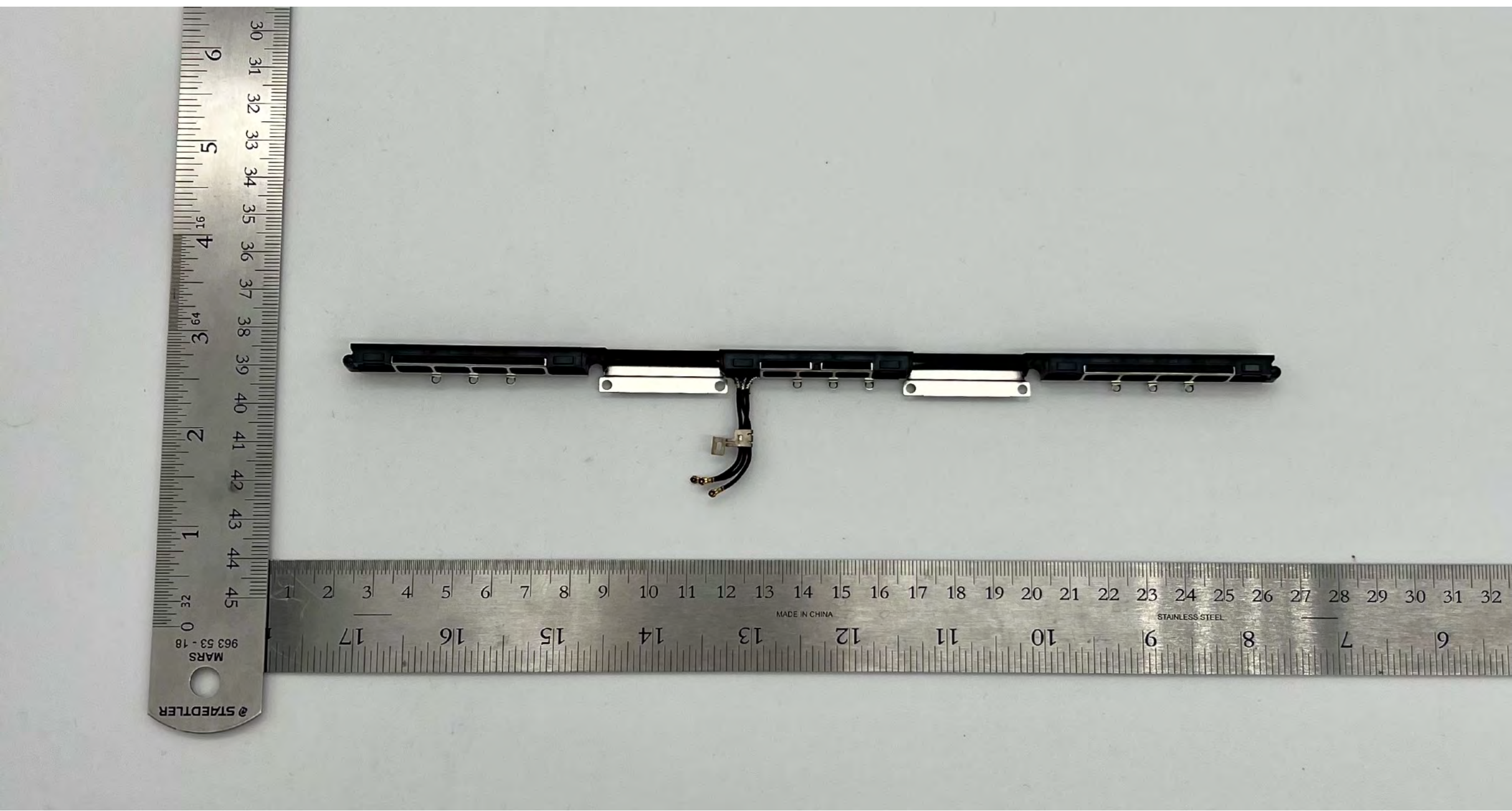
A2779 WF1/BT, WF2/BT, WF3 (BT) antenna structure and feed- Back
