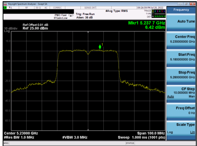
Plot 7-216. PSD Antenna 5b (40MHz BW 802.11ax(SU) – Ch. 46, MCS11)
