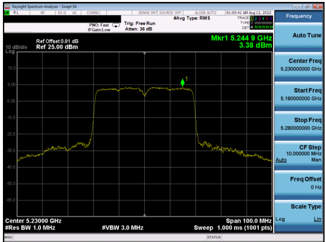
Plot 7-270. ISED PSD Antenna 5b (40MHz BW 11ax(SU) – Ch.46, MCS11)
