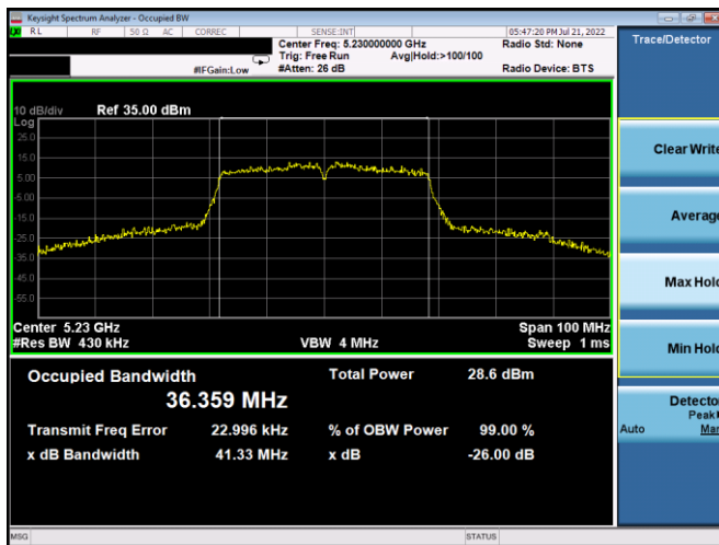
Plot 7-69. 26dB BW & 99% OBW Antenna 4a (40MHz BW 802.11n – Ch. 46, MCS2)
