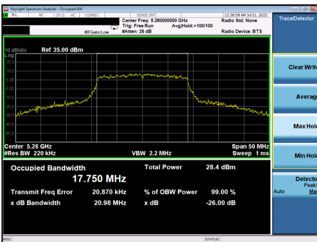
Plot 7-97. 26dB BW & 99% OBW Antenna 4a (20MHz BW 802.11n – Ch. 56, MCS4)
