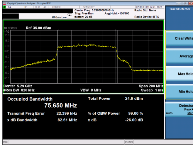
Plot 7-79. 26dB BW & 99% OBW Antenna 4a (80MHz BW 802.11ac – Ch. 58, MCS2)
