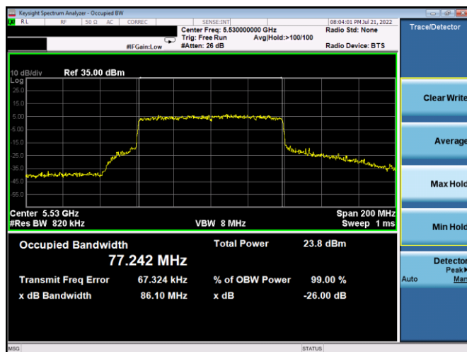
Plot 7-86. 26dB BW & 99% OBW Antenna 4a (80MHz BW 802.11ax(SU) – Ch. 106, MCS2)
