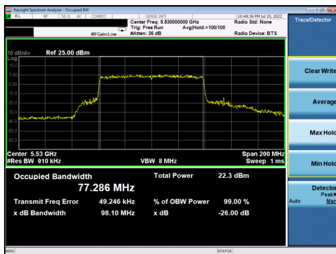
Plot 7-42. 26dB BW & 99% OBW Antenna 5b (80MHz BW 802.11ax(SU) – Ch. 106, MCS4)
