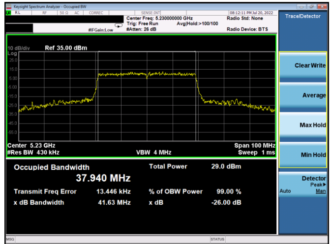
Plot 7-26. 26dB BW & 99% OBW Antenna 5b (40MHz BW 802.11ax(SU) – Ch. 46, MCS4)
