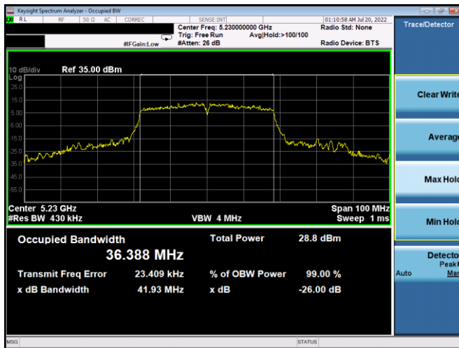
Plot 7-25. 26dB BW & 99% OBW Antenna 5b (40MHz BW 802.11n – Ch. 46, MCS4)
