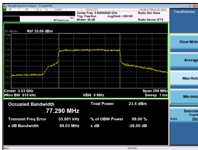
Plot 7-20. 26dB BW & 99% OBW Antenna 5b (80MHz BW 802.11ax(SU) – Ch. 106, MCS2)
