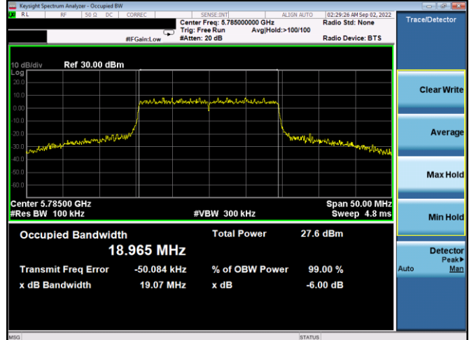
Plot 7-104. 6dB BW & 99% OBW Antenna WF4a (20MHz BW 11ax– RU242 – Ch.157)
