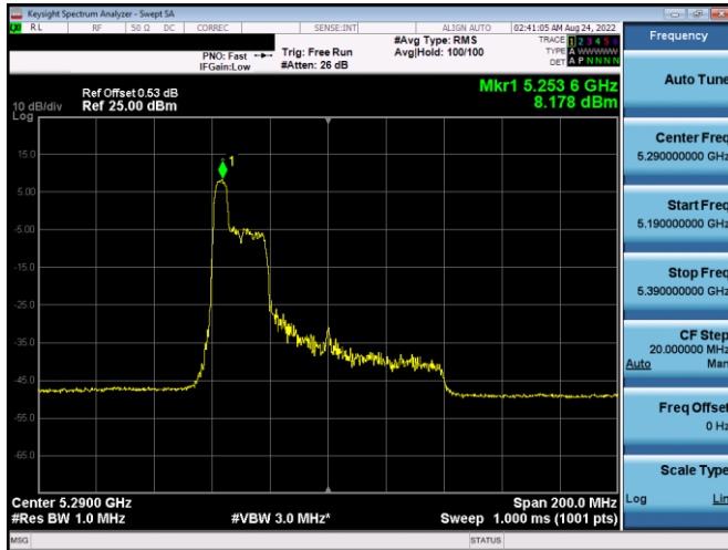
Plot 7-137. PSD Antenna WF5b (80MHz BW 11ax Index 37 - RU52 - Ch.58)
