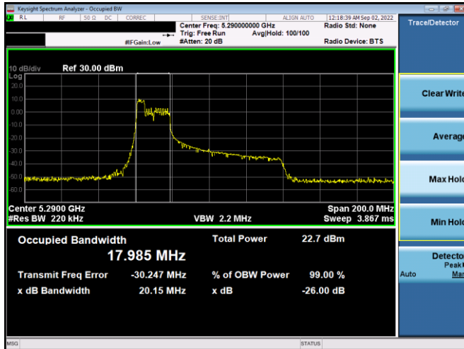
Plot 7-69. 26dB BW & 99% OBW Antenna WF4a (80MHz BW 11ax Index 37 – RU52 – Ch.58)
