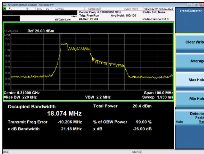
Plot 7-65. 26dB BW & 99% OBW Antenna WF4a (40MHz BW 11ax Index 37 - RU52 - Ch.54)
