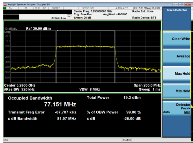
Plot 7-72. 26dB BW & 99% OBW Antenna WF4a (80MHz BW 11ax – RU996 – Ch.58)
