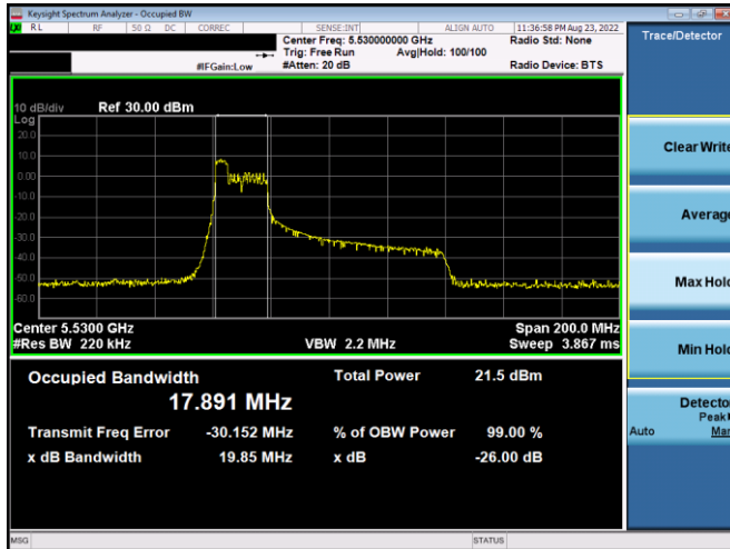
Plot 7-81. 26dB BW & 99% OBW Antenna WF4a (80MHz BW 11ax Index 37 – RU52 – Ch.106)
