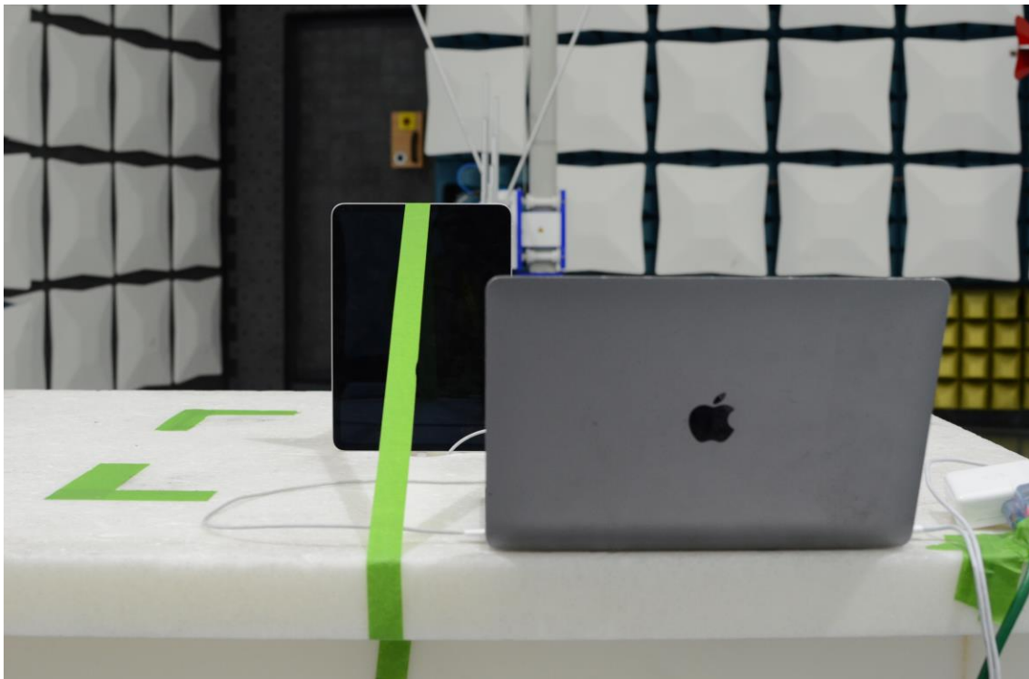
Figure 22: 30MHz-1GHz Test Setup (Rear View)
