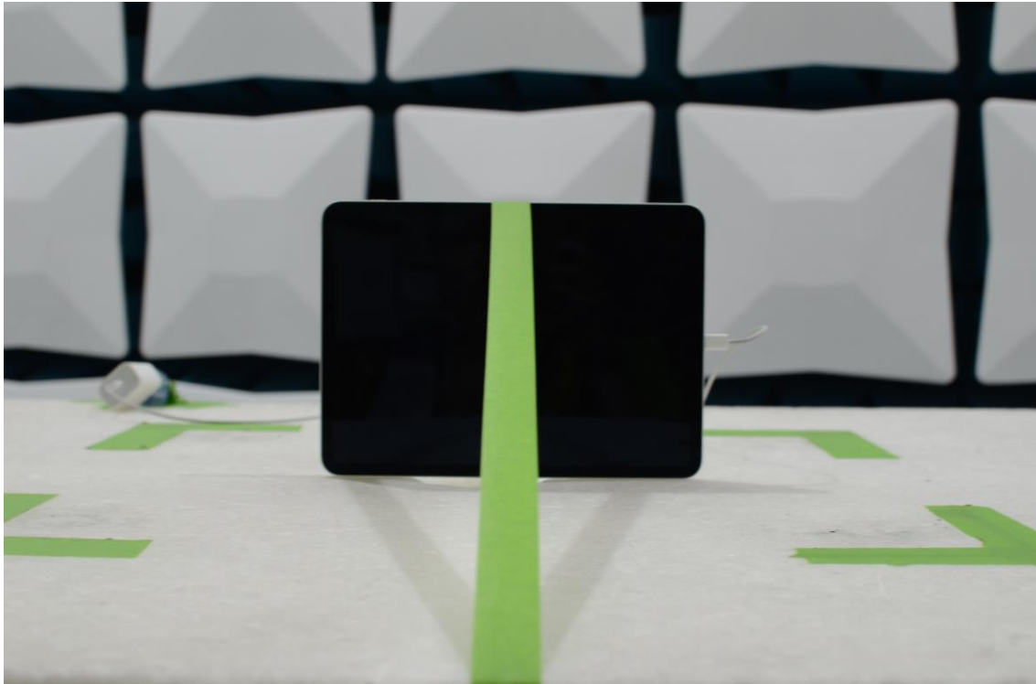
Figure 13: 30MHz-1GHz Test Setup (Front View)
