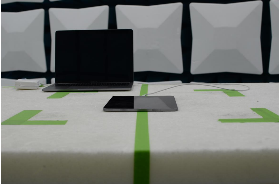
Figure 17: 30MHz-1GHz Test Setup (Front View)
