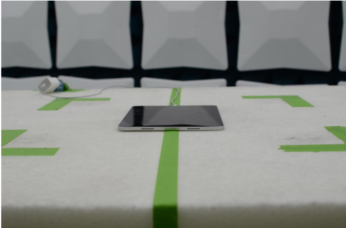
Figure 11: 30MHz-1GHz Test Setup (Front View)
