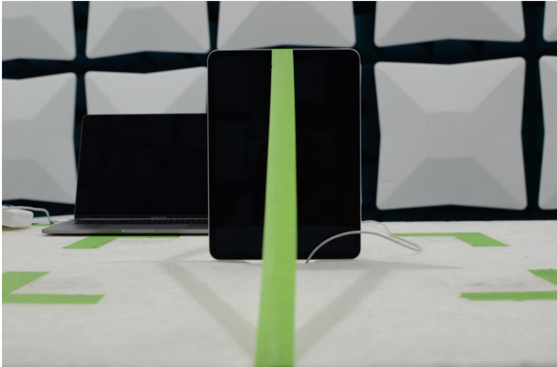
Figure 21: 30MHz-1GHz Test Setup (Front View)
