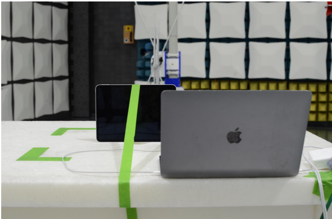
Figure 20: 30MHz-1GHz Test Setup (Rear View)
