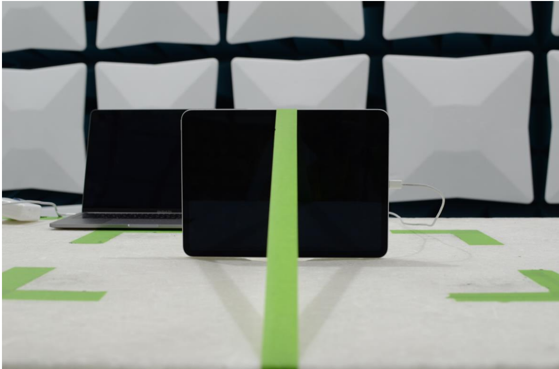
Figure 19: 30MHz-1GHz Test Setup (Front View)
