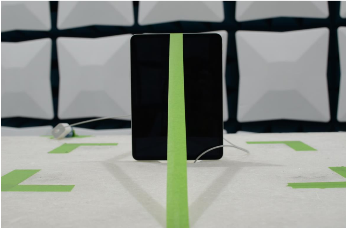
Figure 15: 30MHz-1GHz Test Setup (Front View)
