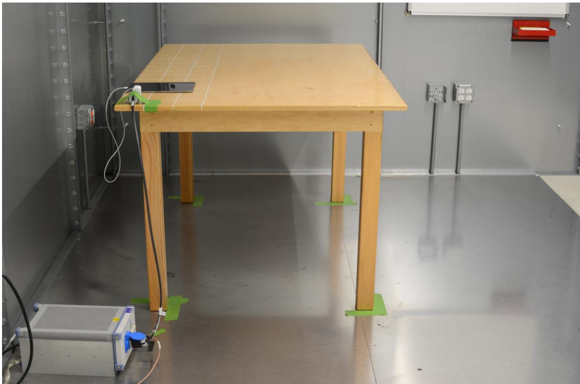
Figure 2: AC Line Conducted Emissions (Side View)
