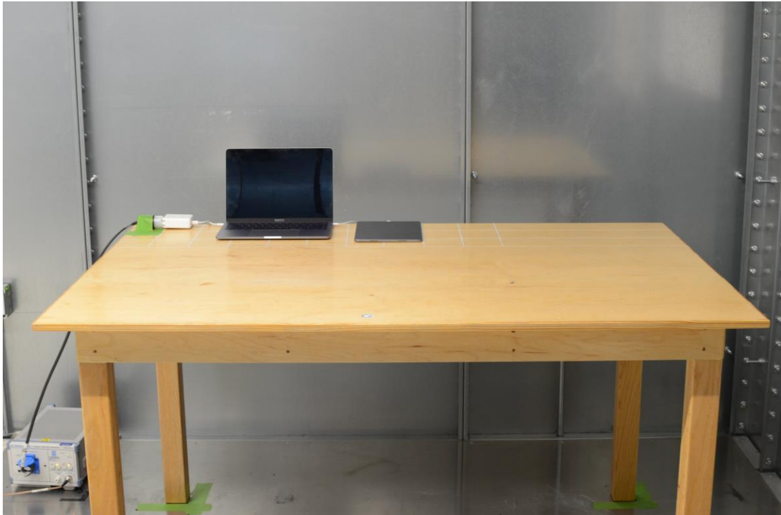
Figure 3: AC Line Conducted Emissions (Front View)
