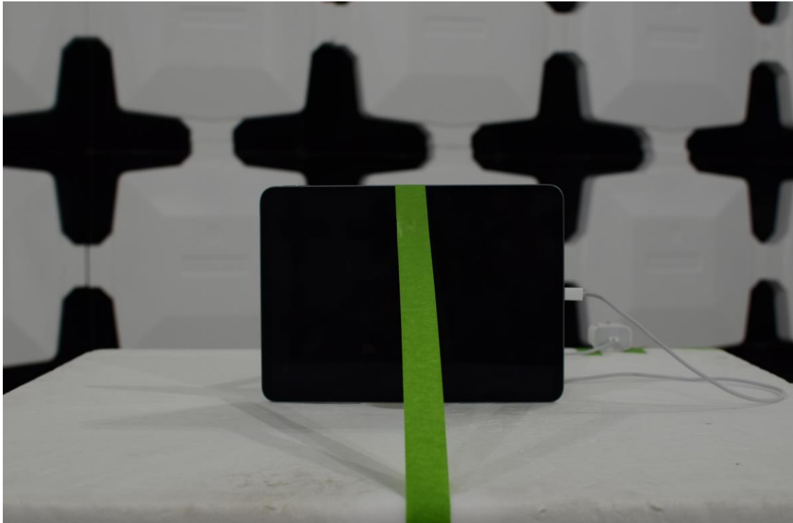
Figure 7: 1-18GHz Test Setup (Front View)
