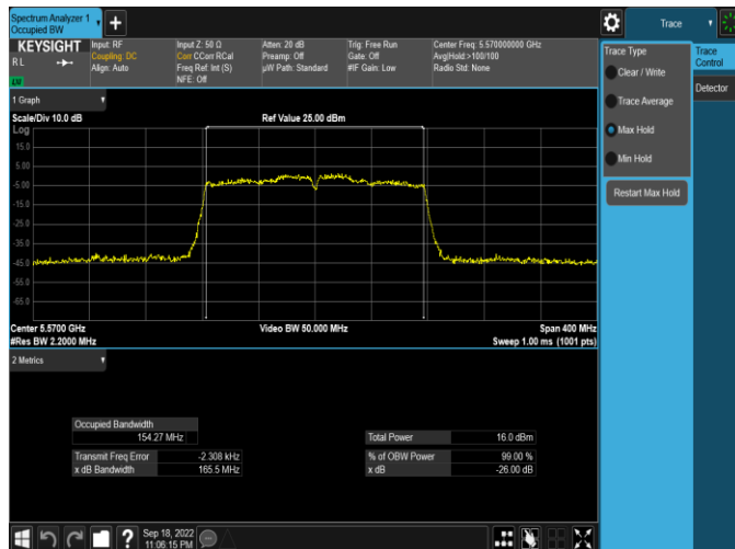
Plot 7-21. 26dB BW & 99% OBW Antenna WF5T (160MHz BW 802.11ac – Ch. 114, MCS2)
