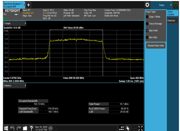
Plot 7-22. 26dB BW & 99% OBW Antenna WF5T (160MHz BW 802.11ax(SU) – Ch. 114, MCS2)
