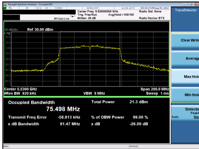
Plot 7-19. 26dB BW & 99% OBW Antenna WF5T (80MHz BW 802.11ac – Ch. 106, MCS2)
