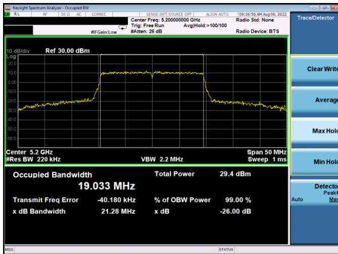
Plot 7-24. 26dB BW & 99% OBW Antenna WF5T (20MHz BW 802.11ax(SU) – Ch. 40, MCS4)
