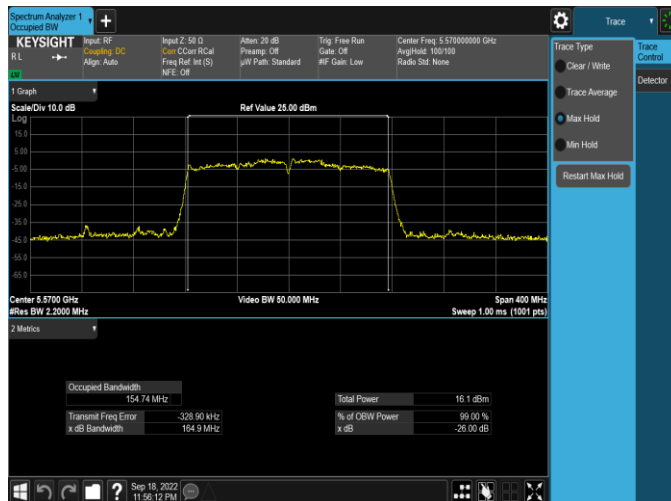
Plot 7-43. 26dB BW & 99% OBW Antenna WF5T (160MHz BW 802.11ac – Ch. 114, MCS4)
