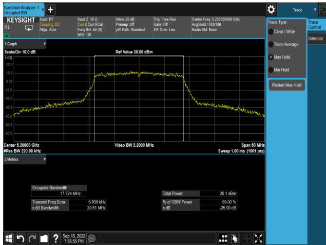
Plot 7-23. 26dB BW & 99% OBW Antenna WF5T (20MHz BW 802.11n – Ch. 40, MCS4)
