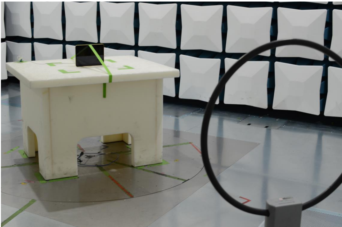
Figure 20: 9kHz-30MHz Test Setup (Front View)
