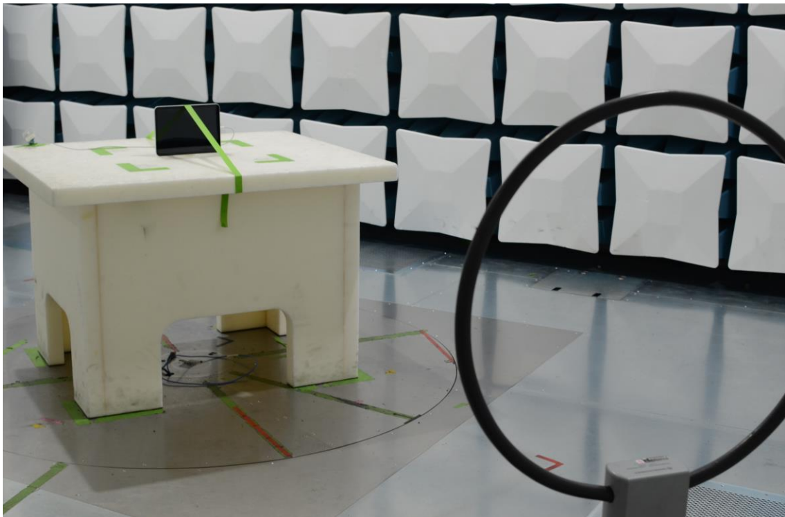
Figure 24: 9kHz-30MHz Test Setup (Front View)
