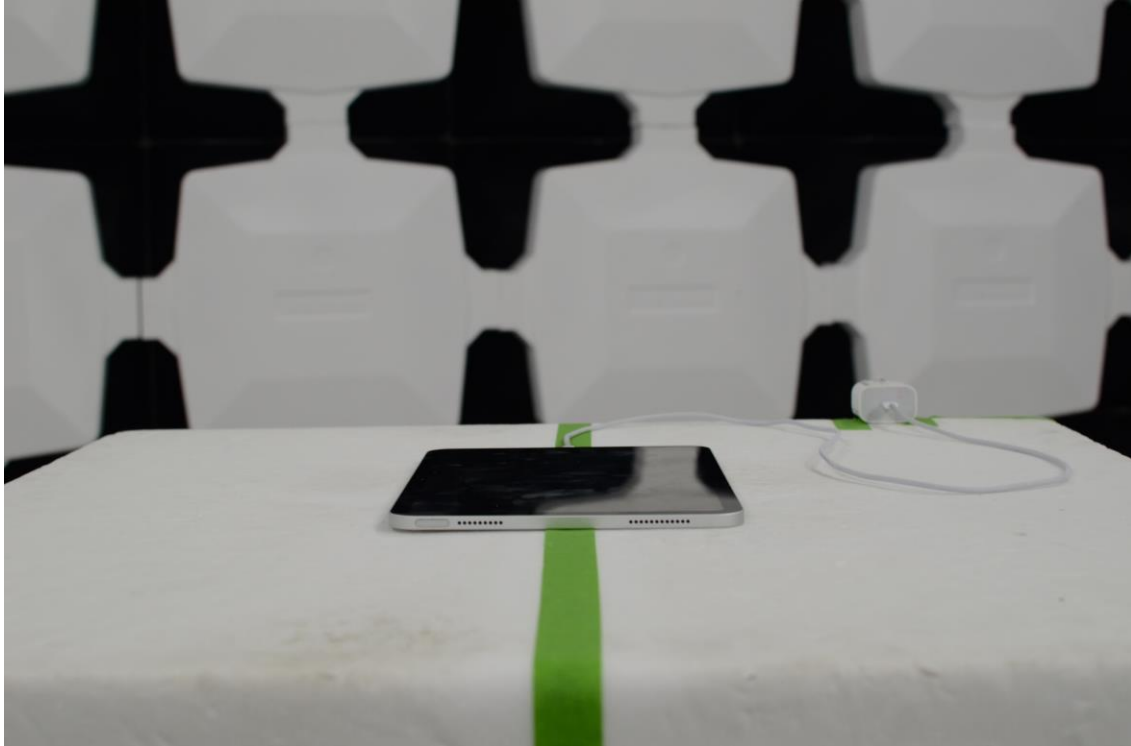
Figure 5: 1-18GHz Test Setup (Front View)
