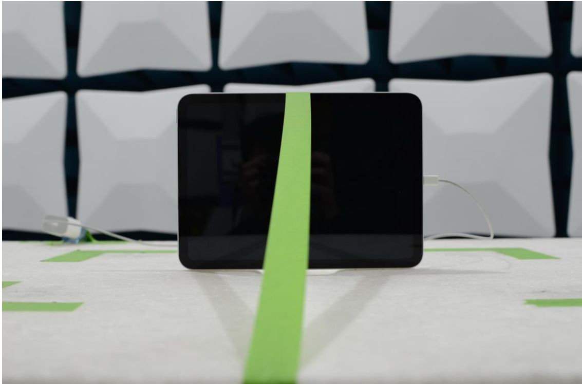
Figure 13: 30MHz-1GHz Test Setup (Front View)
