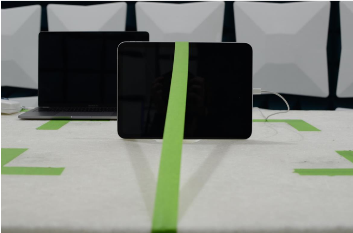
Figure 19: 30MHz-1GHz Test Setup (Front View)
