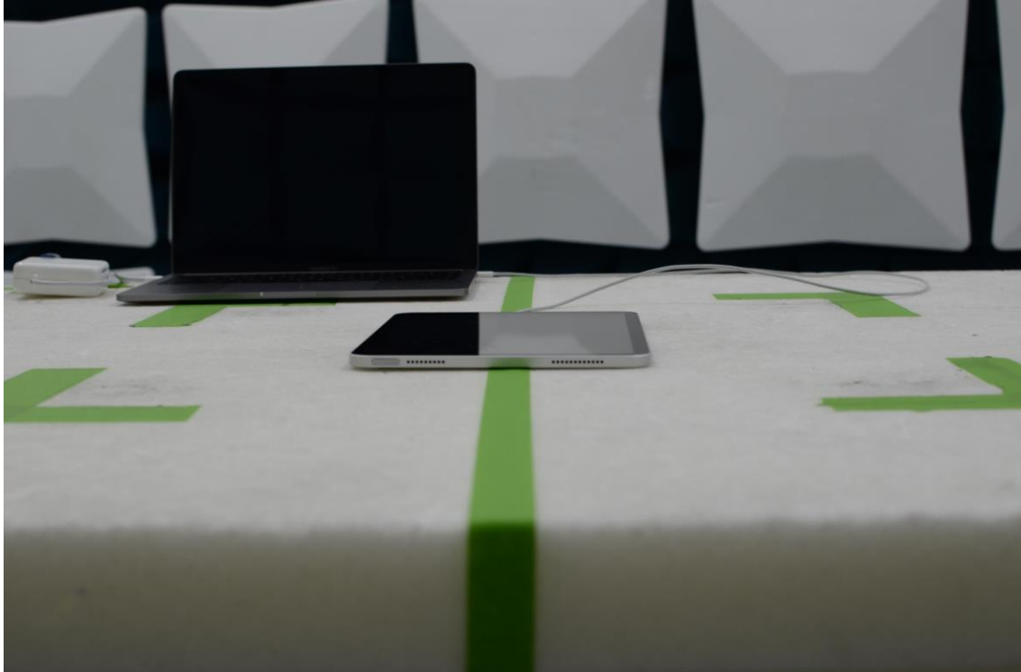
Figure 17: 30MHz-1GHz Test Setup (Front View)
