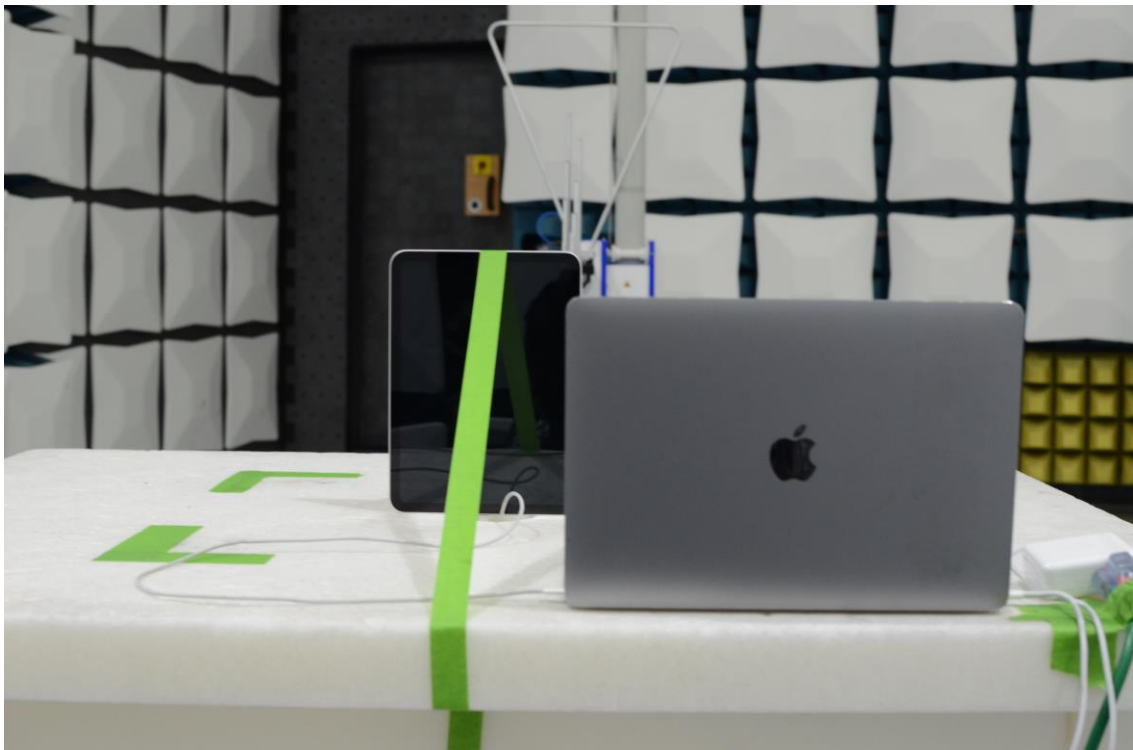
Figure 22: 30MHz-1GHz Test Setup (Rear View)
