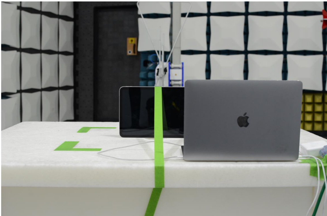
Figure 20: 30MHz-1GHz Test Setup (Rear View)
