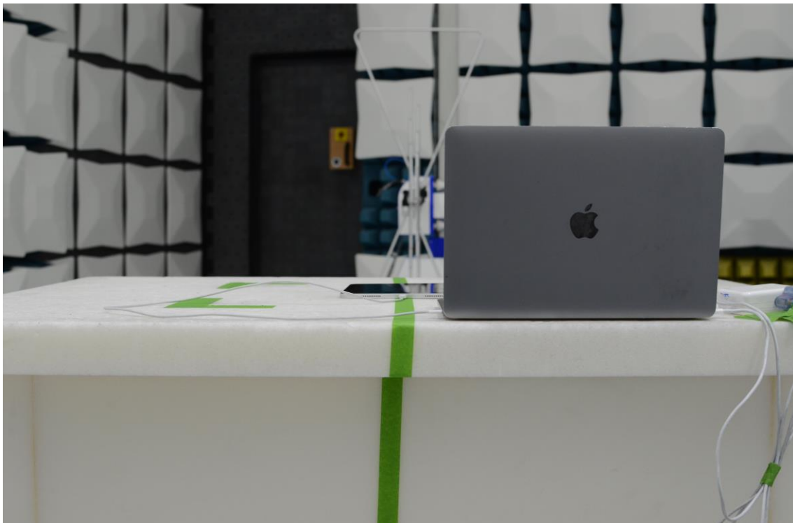
Figure 18: 30MHz-1GHz Test Setup (Rear View)
