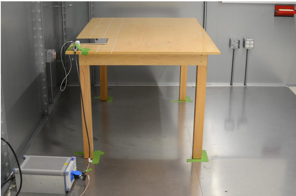
Figure 2: AC Line Conducted Emissions (Side View)
