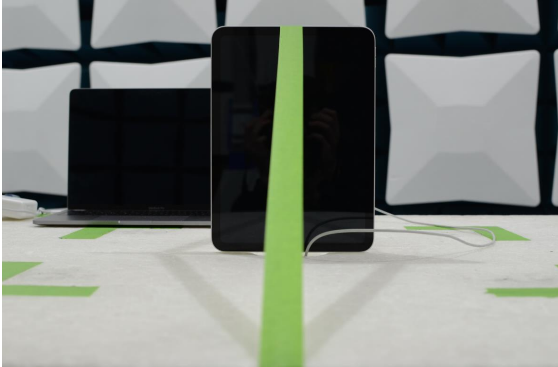
Figure 21: 30MHz-1GHz Test Setup (Front View)
