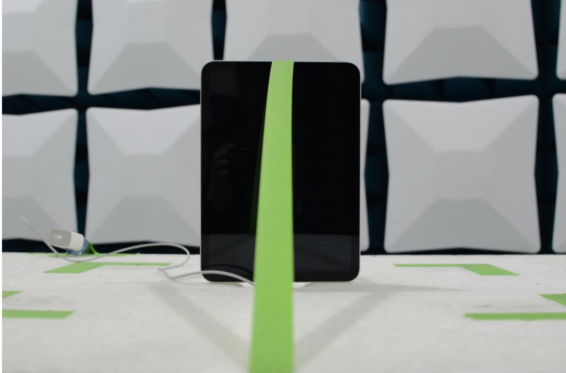
Figure 15: 30MHz-1GHz Test Setup (Front View)
