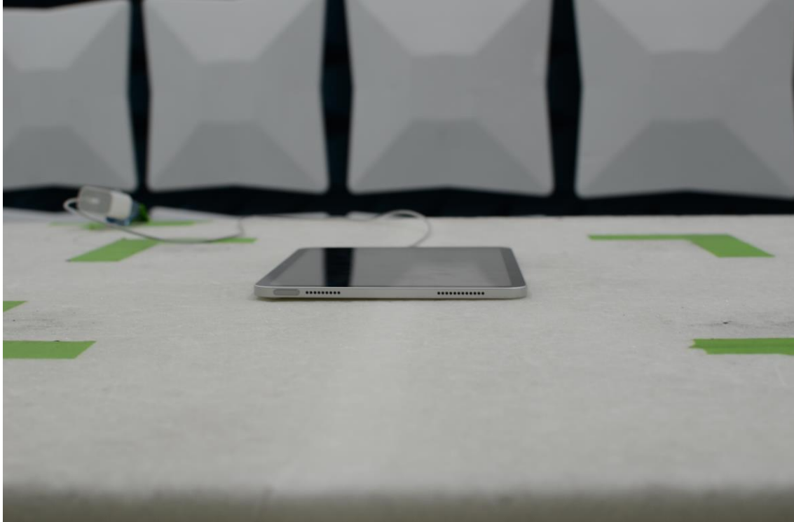
Figure 11: 30MHz-1GHz Test Setup (Front View)
