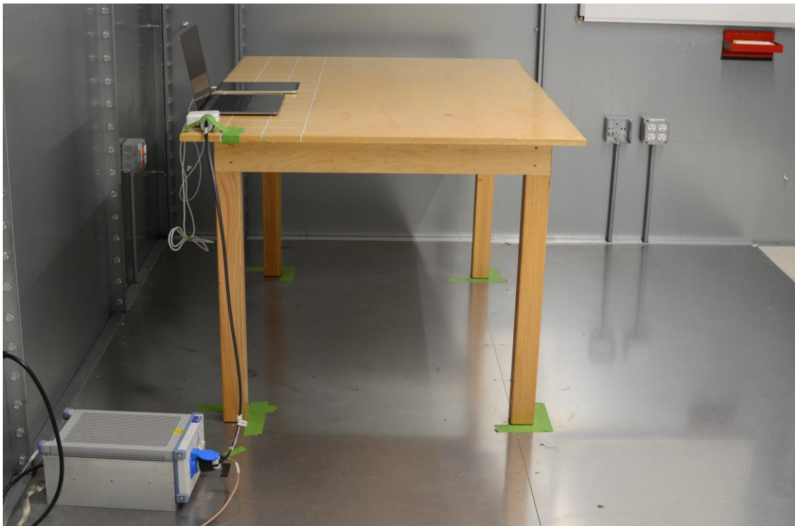
Figure 4: AC Line Conducted Emissions (Side View)
