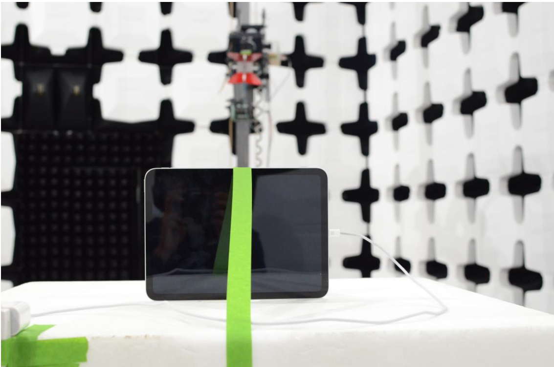
Figure 8: 1-18GHz Test Setup (Rear View)
