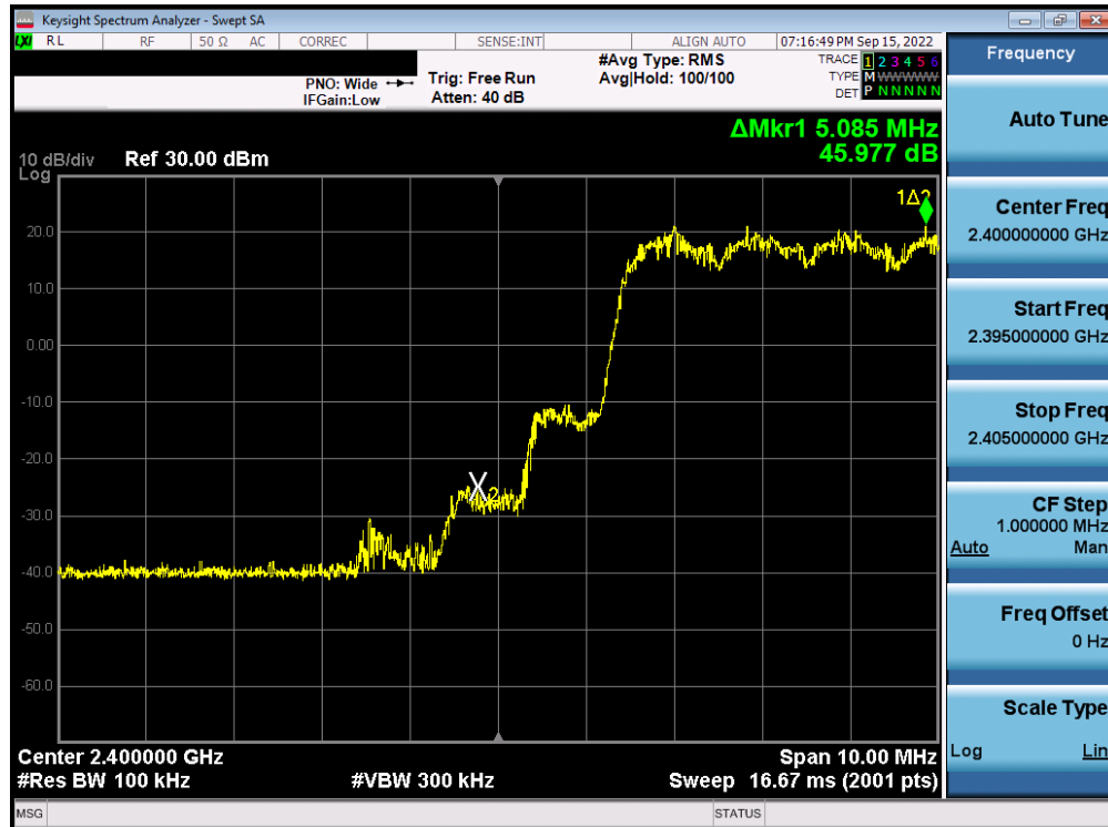
Plot 7-27. Band Edge Plot Antenna WF7b (Bluetooth with Hopping Enabled, 8DPSK, ePA)
