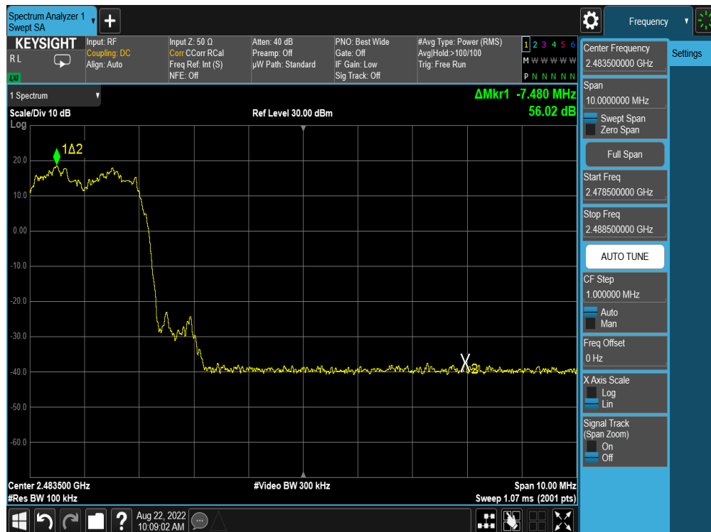
Plot 7-20. Band Edge Plot Antenna WF8 (Bluetooth with Hopping Enabled, 8DPSK, ePA)
