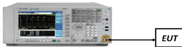
Figure 7-1. Test Instrument & Measurement Setup
