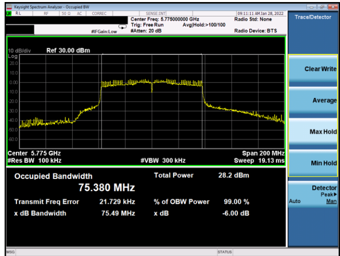
Plot 7-113. 6dB BW & 99% OBW Antenna WF8 (80MHz BW 802.11ac – Ch. 155, MCS0)
