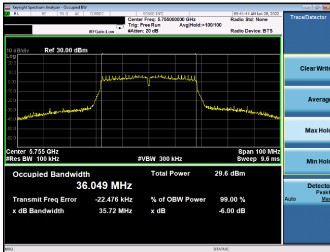
Plot 7-129. 6dB BW & 99% OBW Antenna WF7a (40MHz BW 802.11n – Ch. 151, MCS0)
