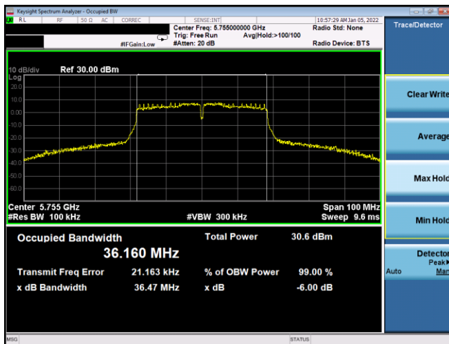
Plot 7-117. 6dB BW & 99% OBW Antenna WF8 (40MHz BW 802.11n – Ch. 151, MCS3)
