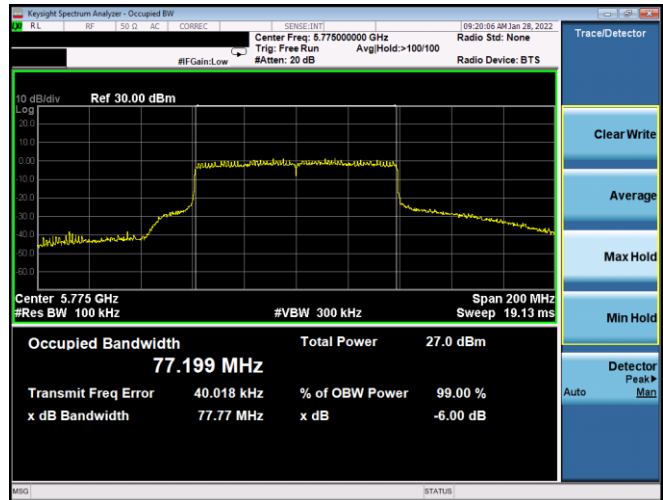
Plot 7-114. 6dB BW & 99% OBW Antenna WF8 (80MHz BW 802.11ax(SU) – Ch. 155, MCS0)
