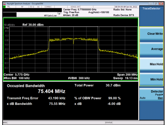
Plot 7-119. 6dB BW & 99% OBW Antenna WF8 (80MHz BW 802.11ac – Ch. 155, MCS3)
