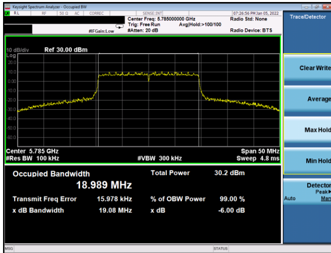
Plot 7-122. 6dB BW & 99% OBW Antenna WF8 (20MHz BW 802.11ax(SU) – Ch. 157, MCS5)
