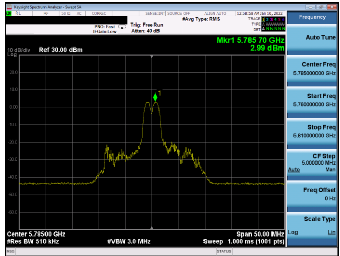
Plot 7-292. PSD CDD Antenna WF7a (20MHz BW 11ax Index 4 – RU26 – Ch.157)
