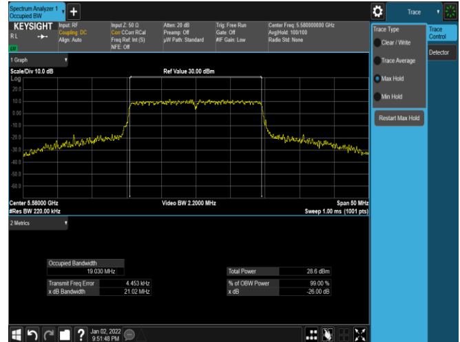
Plot 7-28. 26dB BW & 99% OBW Antenna WF8 (20MHz BW 11ax– RU242 – Ch.116)
