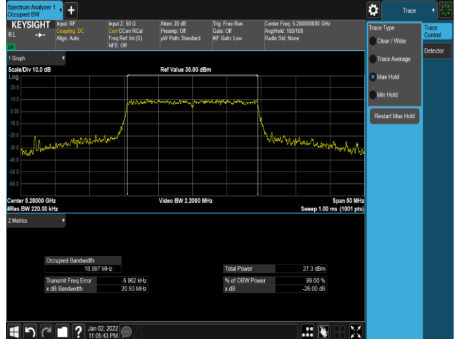
Plot 7-52. 26dB BW & 99% OBW Antenna WF7a (20MHz BW 11ax – RU242 – Ch.56)
