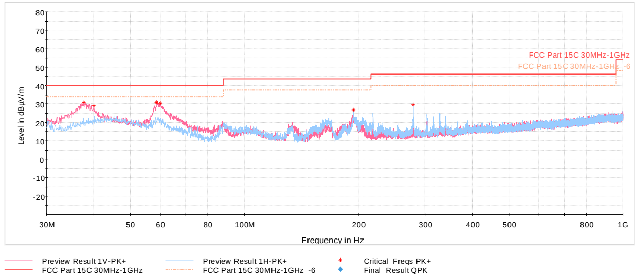
Plot 7-1878. Radiated Spurious Emissions below 1GHz CDD/SDM Diversity, 802.11ax (SU), Ch.36 with AC/DC Adapter
