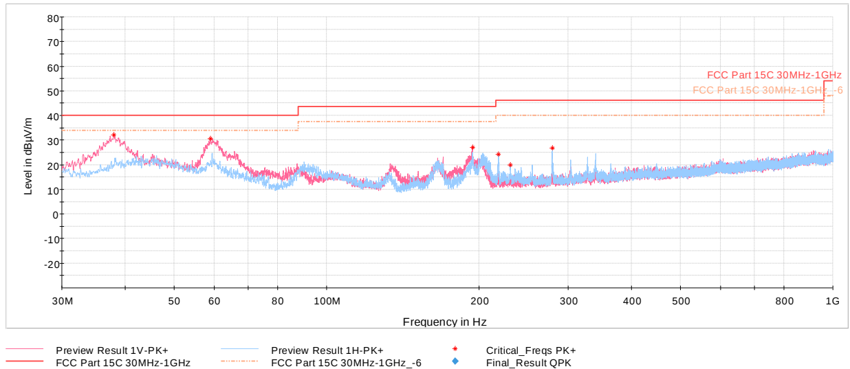
Plot 7-1877. Radiated Spurious Emissions below 1GHz CDD/SDM Diversity, 802.11n, Ch.36 with AC/DC Adapter
