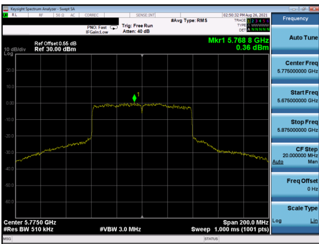
Plot 7-456. PSD Antenna 1b (80MHz BW 802.11ax(SU) – Ch. 155, MCS2)
