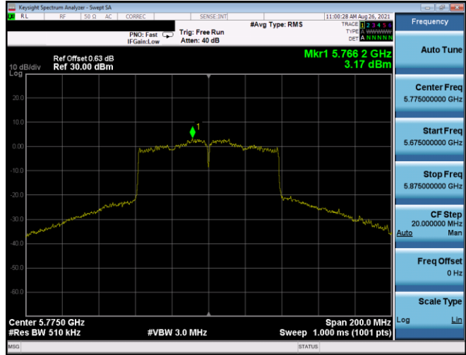
Plot 7-281. PSD Antenna 5T (80MHz BW 802.11ac – Ch. 155, MCS3)
