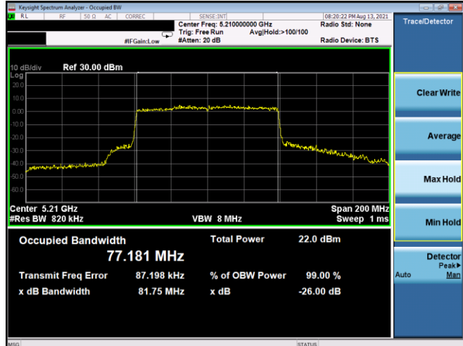
Plot 7-132. 26dB BW & 99% OBW Antenna 1b (80MHz BW 802.11ax(SU) – Ch. 42, MCS3)
