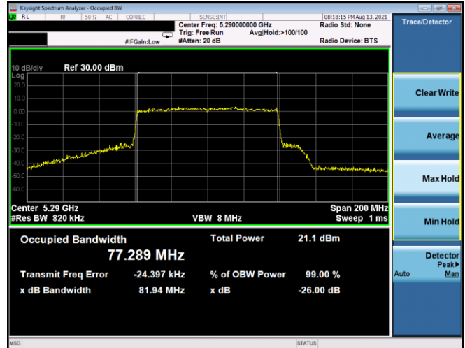
Plot 7-138. 26dB BW & 99% OBW Antenna 1b (80MHz BW 802.11ax(SU) – Ch. 58, MCS3)
