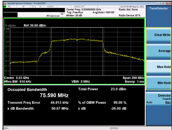
Plot 7-71. 26dB BW & 99% OBW Antenna 3b (80MHz BW 802.11ax(SU) – Ch. 106, MCS2)
