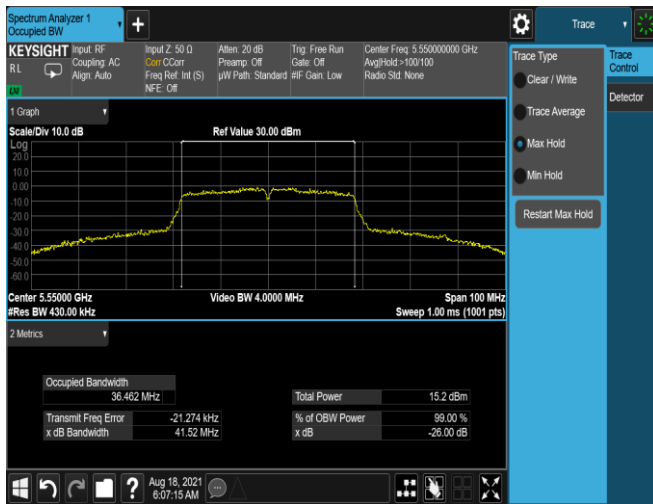
Plot 7-87. 26dB BW & 99% OBW Antenna 3b (40MHz BW 802.11n – Ch. 110, MCS3)
