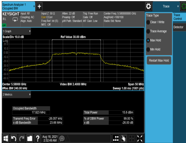
Plot 7-85. 26dB BW & 99% OBW Antenna 3b (20MHz BW 802.11n – Ch. 116, MCS3)
