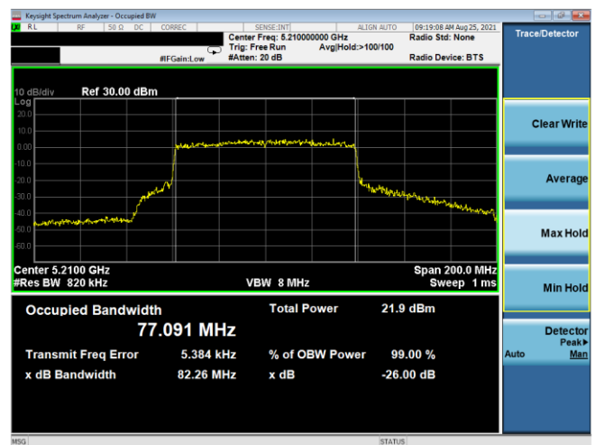
Plot 7-60. 26dB BW & 99% OBW Antenna 3b (80MHz BW 802.11ax(SU) – Ch. 42, MCS2)
