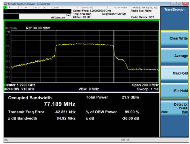
Plot 7-66. 26dB BW & 99% OBW Antenna 3b (80MHz BW 802.11ax(SU) – Ch. 58, MCS2)
