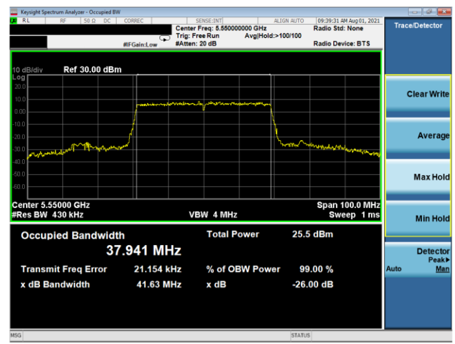
Plot 7-70. 26dB BW & 99% OBW Antenna 3b (40MHz BW 802.11ax(SU) – Ch. 110) , MCS2)
