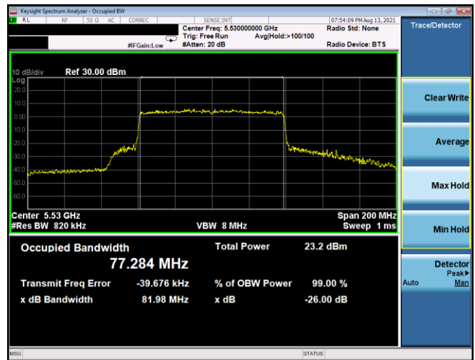
Plot 7-90. 26dB BW & 99% OBW Antenna 3b (80MHz BW 802.11ax(SU) – Ch. 106, MCS3)
