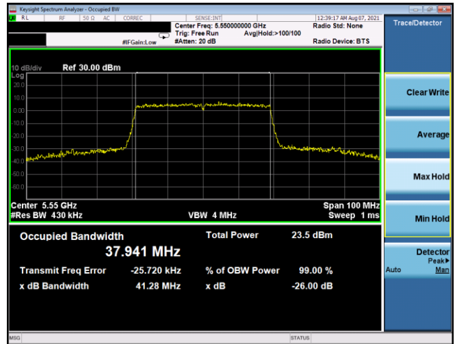
Plot 7-88. 26dB BW & 99% OBW Antenna 3b (40MHz BW 802.11ax(SU) – Ch. 110, MCS3)
