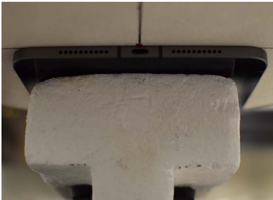
Test Setup Photo 6 – Back Side Antenna 1b, and 2 SAR at 0 mm
