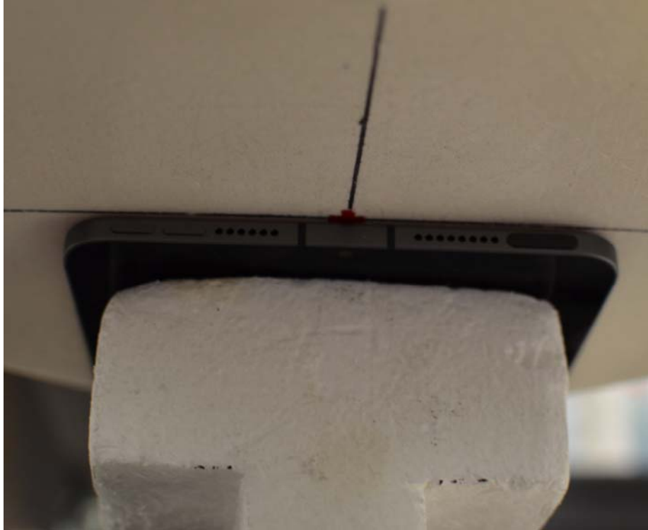
Test Setup Photo 7 – Back Side Antenna 4 SAR at 0 mm
