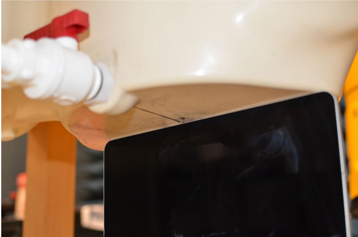
SAR Test Setup Photo 6: Right Edge at 0.0 cm – Ant 4a/4b/3
