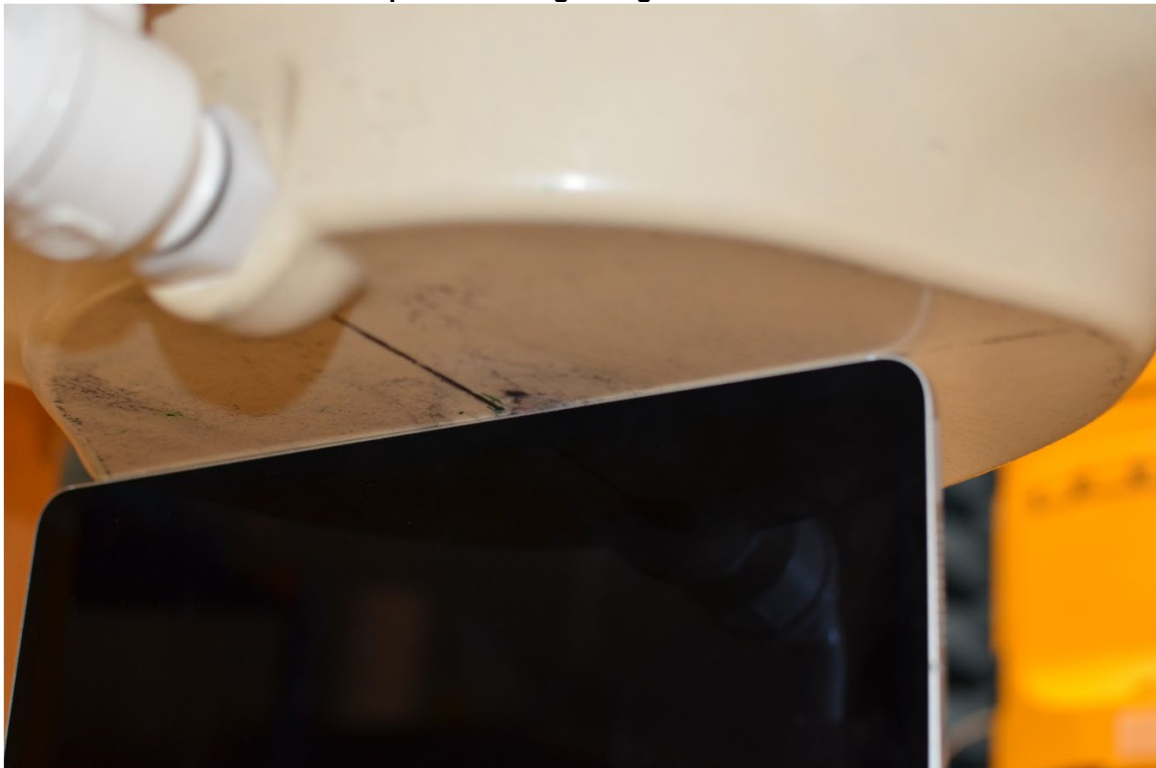
SAR Test Setup Photo 7: Right Edge at 0.0 cm – Ant 2a/2b/1/5b
