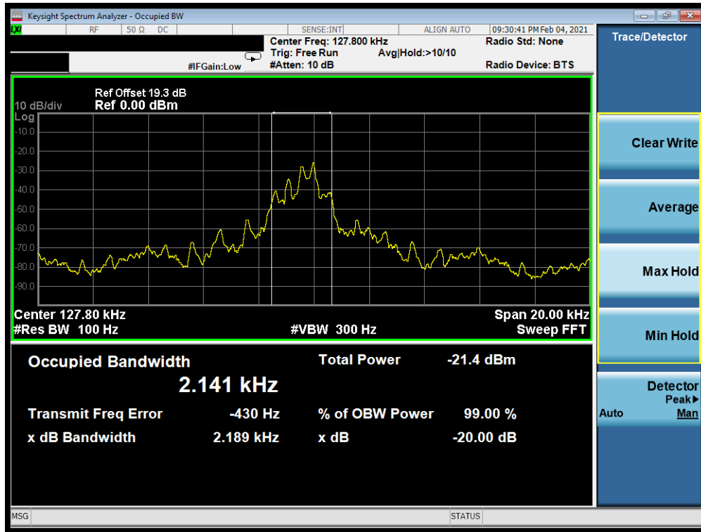
Plot 6-1. Occupied Bandwidth Plot (Charging Rate 10C)
