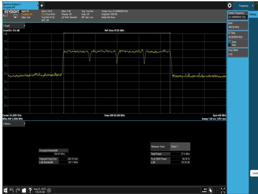
Plot 7-49. Ant M0 OBW (Band n258-R1-50MHz-4CC SISO DFTs-OFDM – 64QAM – Mid Channel)
