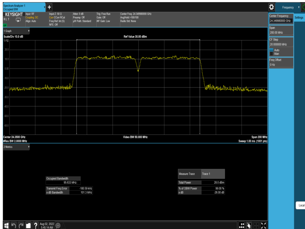
Plot 7-20. Ant M0 OBW (Band n258-R1-50MHz-2CC SISO DFTs-OFDM – 16QAM – Mid Channel)
