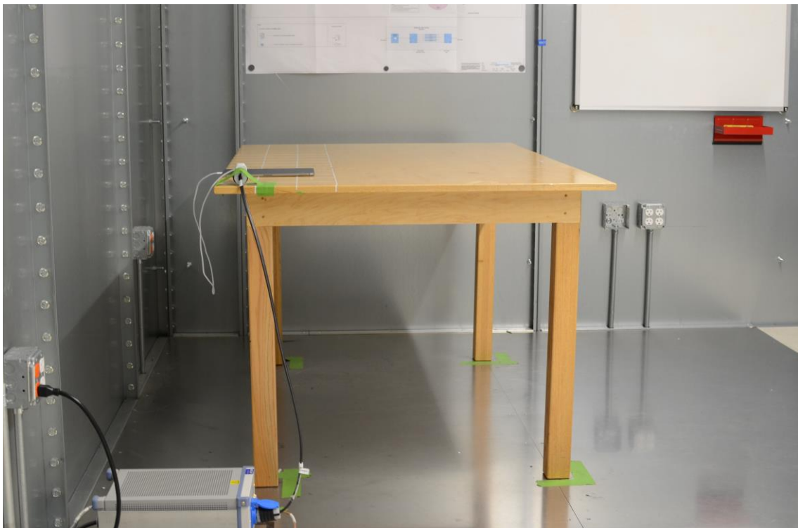
Figure 2: AC Line Conducted Emissions (Side View)
